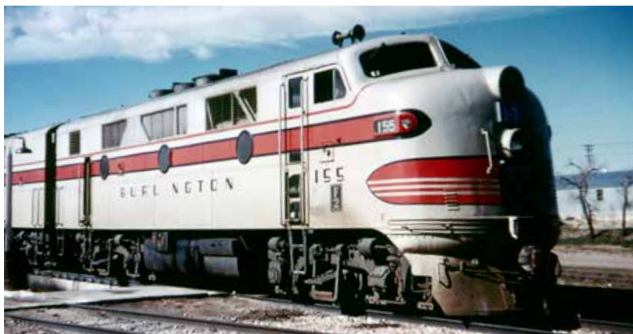
The F2 was produced briefly in 1946 while EMD developed a 1,500-h.p.-capable generator for the F3. Although much advanced over the FT, the F2 retained the FT's 1,350 h.p. rating. K. C. Crist
