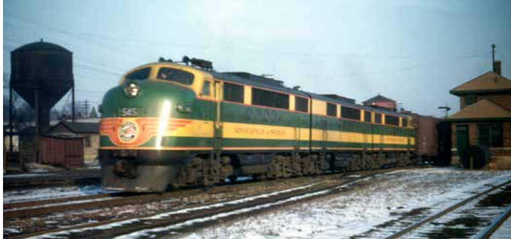
Minneapolis & St. Louis 545 catches a bit of sun at Marshalltown, Iowa, on November 9, 1947. The drawbar-connected A-B-A set was half of M&StL's FT fleet. D. Christensen; F. and T. Novak coll.
