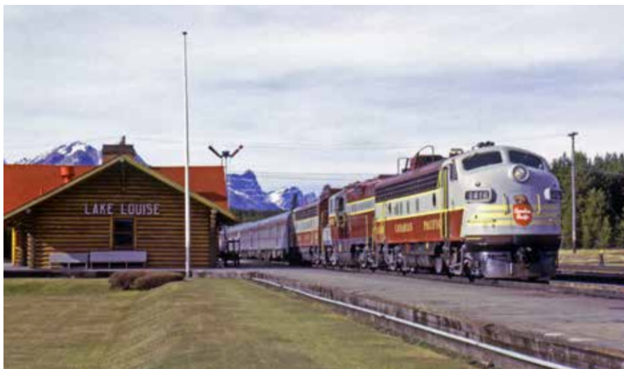
Canadian Pacific 1416 leads an FP7-GP9-FP7 consist on the eastbound Canadian at Lake Louise, Alberta, in October 1964. All 83 of CP's Fs were bought for passenger duty. James A. Brown
