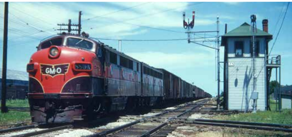
Gulf, Mobile & Ohio had 12 dual-service F3s (9 As, 3 Bs), some ordered by the Alton; No. 880A leads a southbound freight across IC and IT tracks at Athol Tower in Lincoln, Ill., in July 1952. Rebuilt, this unit worked into the 2000s on Metro-North. George Krambles, Krambles-Peterson Archive
