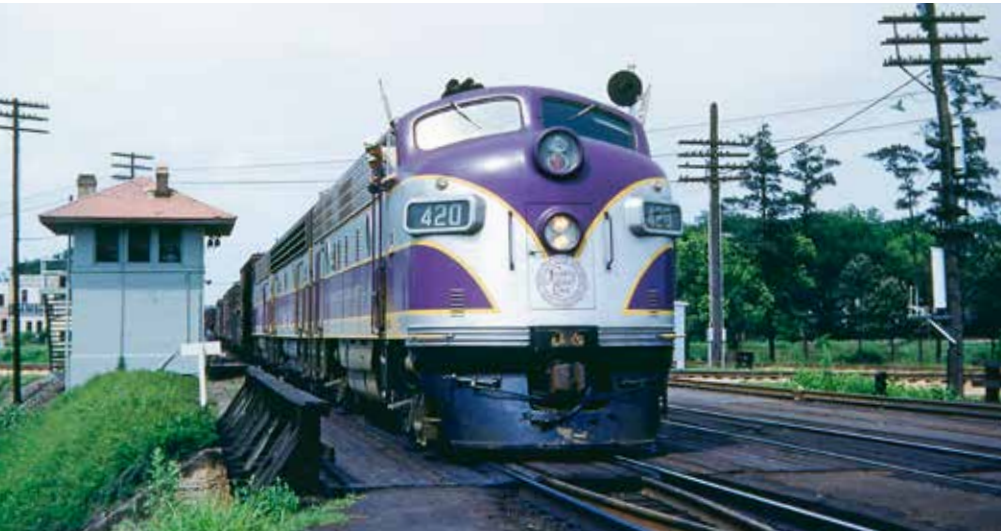
Nearly new Atlantic Coast Line F7 420 leads an A-B-A consist on a freight extra south over the Norfolk Southern Railway crossing at Fayetteville, N.C., in spring 1952. EMD-oriented Coast Line had 230 F units of models FT, 2, 3, 7, 9, and FP7. Robert A. Caflisch, Helen Caflisch coll.
