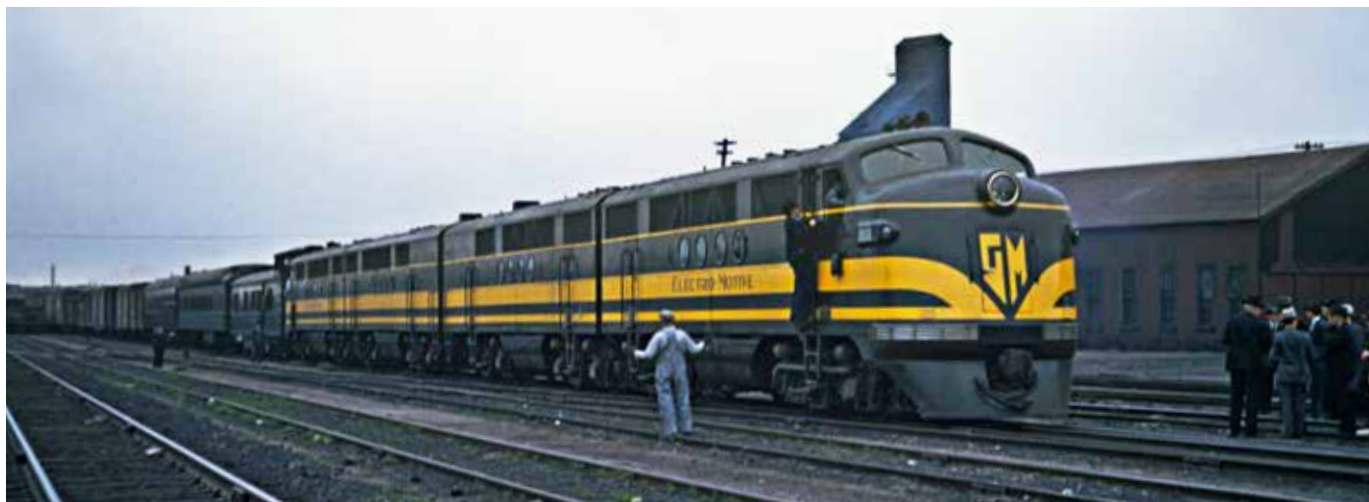
Four-unit FT demonstrator No. 103 is at Denver with test cars and a freight on April 28, 1940, halfway through its nationwide tour. R. H. Kindig
