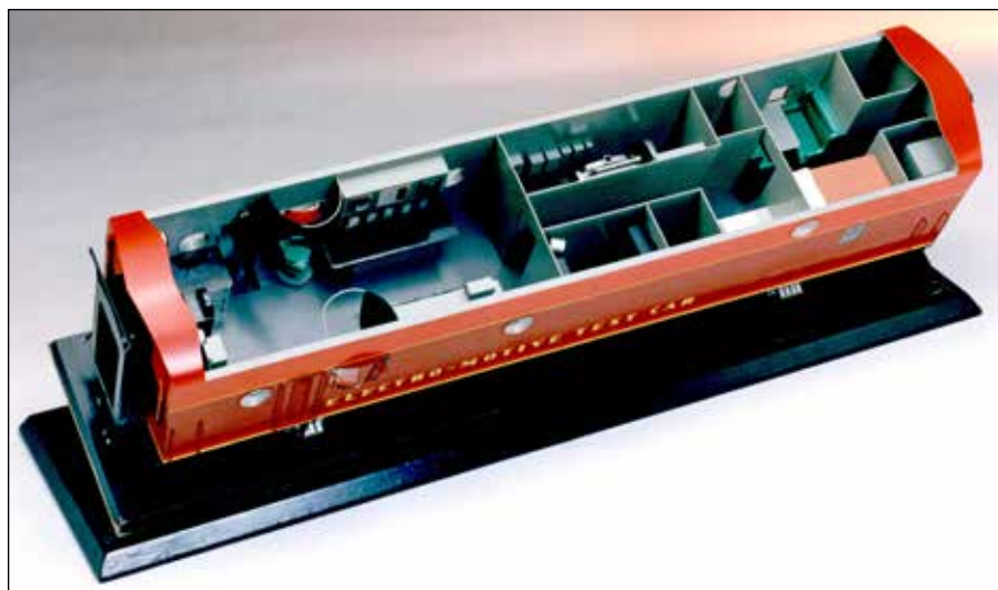
A model of EMD's F-unit-based test car ET-909 shows the monitoring area with small bay windows at one end (left in photo) and crew quarters in the other. EMD, Preston Cook collection
