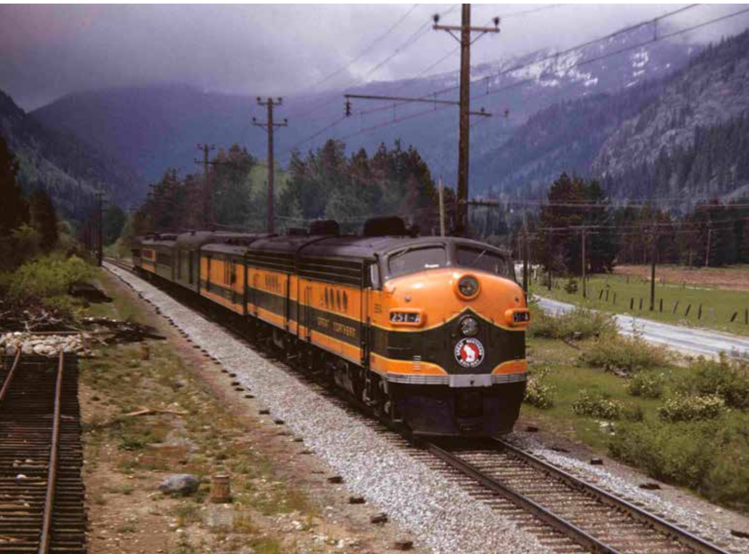
Great Northern FT A-B set 251 heads the Seattle–Spokane (Wash.) Cascadian over Stevens Pass in May 1953. The FTs have been modified with F7-style grilles and large number boxes. At 96 units, GN's FT fleet trailed only Santa Fe's in size. George Krambles, Krambles-Peterson Archive
