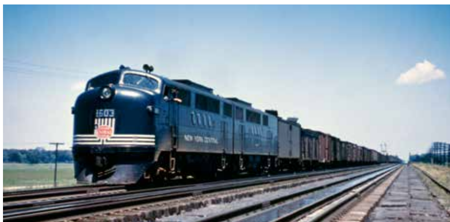
New York Central 1603, the last of the road's four FT A-B sets, ignores the steam locomotive track pans at Stryker, Ohio, as it rolls west with a freight in the late 1940s. Emery Gulash
