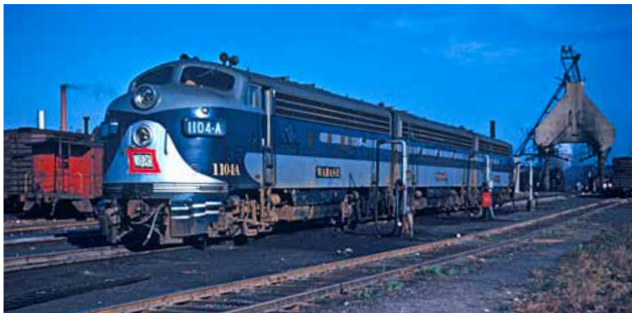
Wabash relied heavily on F7s, trying 9 A-B-A sets in 1949 (one poses brand-new at Montpelier, Ohio), then going for 54 F7A pairs, 22 built in Canada. Barney L. Stone, Krambles-Peterson Archive
