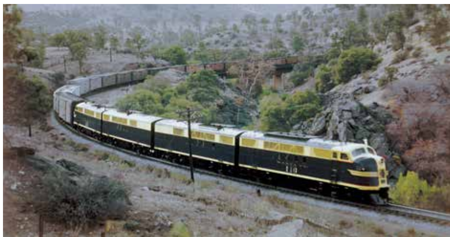
Seven-year-old Santa Fe FTs led by A unit No. 110 employ dynamic braking as they descend California's famous Tehachapi grade with Bay Area-bound freight in 1949. Linn H. Westcott
