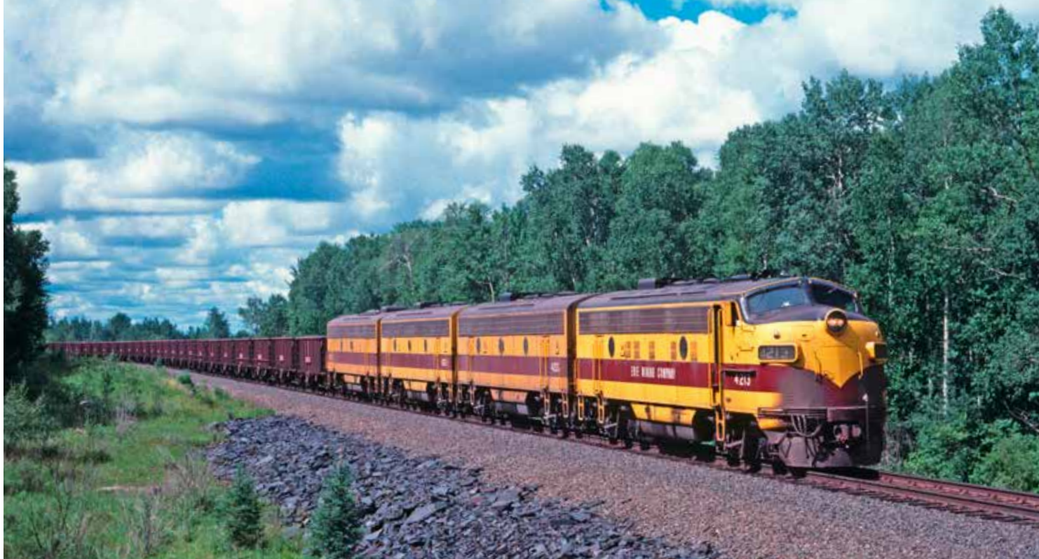
Eleven new F9s worked Erie Mining's 70-mile iron-ore railroad in northern Minnesota when it opened in 1957, and some were still on the job when regular operations ended more than 40 years later. An A-B-B-B consist hauls loads toward Lake Superior in July 1988. Steve Glischinski
