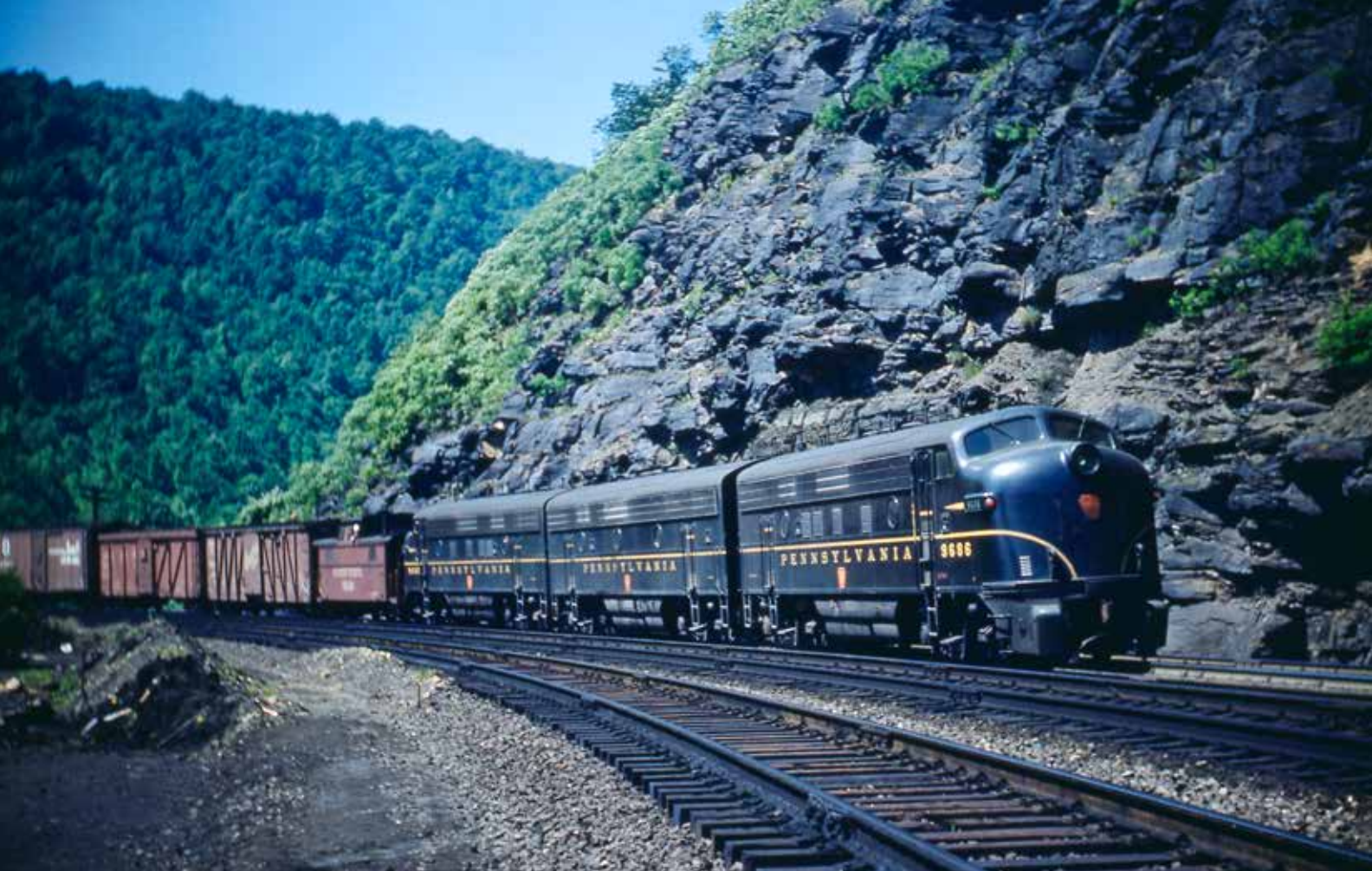
During 1948–50, Pennsy bought 69 F3s and F7s in A-B-A sets for helper service west of Altoona, Pa. The F3s had F7-style side panels, and all the As had PRR-specified small number boxes. On June 19, 1951, an F3 trio assists a 105-car freight up Horseshoe Curve. Edward Theisinger
