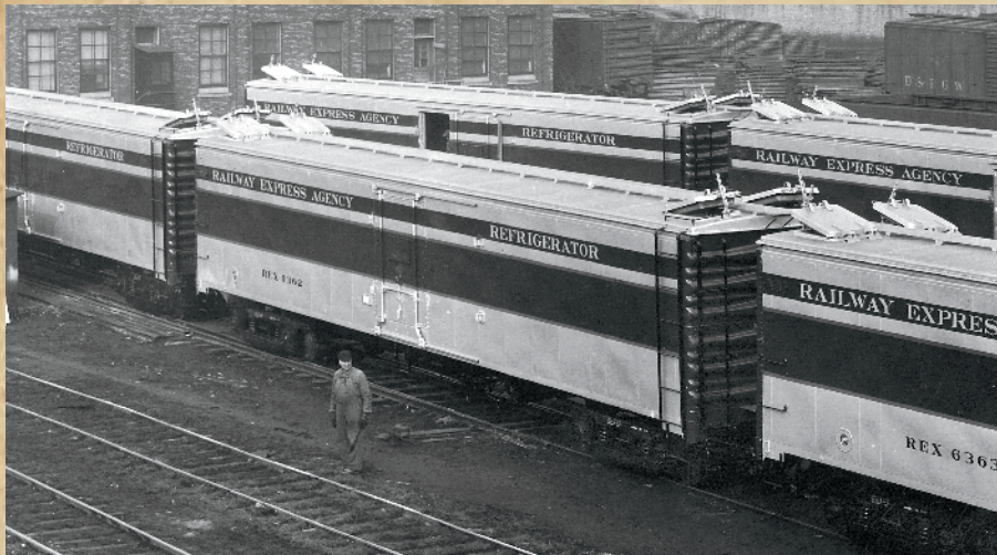
American Car & Foundry built 500 new 55-foot express refrigerator cars for REA in 1947-48. The ice-bunker cars were initially painted aluminum and green as shown here. ACF
