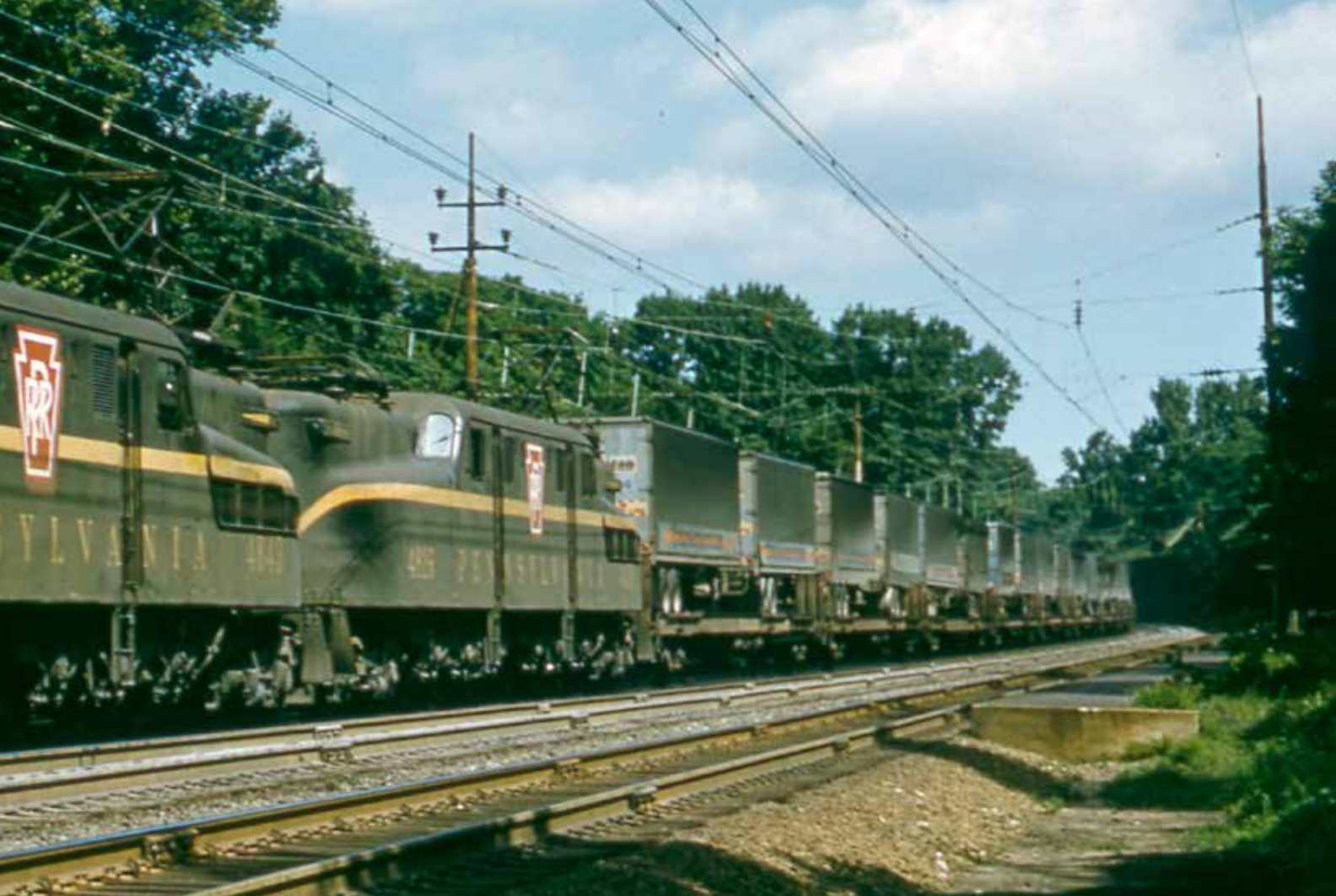
Motors 4843 and 4826, two of PRR's 139 versatile GG1s, head Transamerica piggyback trailers east at Merion in August 1961. Track 3, the westbound freight track, is white with sand dust from trains climbing the hill.
