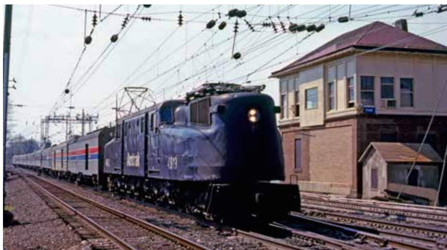
Amtrak GG1 4919 passes Paoli tower with train 40, the eastbound Broadway Limited , New York section, on April 20, 1980, a week before the end of GG1 usage west of Philadelphia. Note the tower’s new brickwork and windows, repairs made after a 1974 freight derailment.
