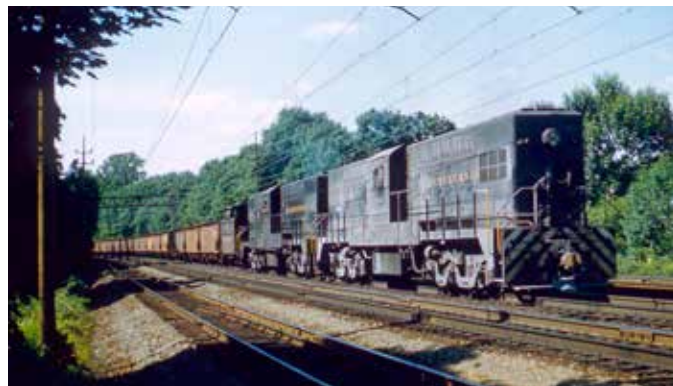
Two 2,400 h.p. Baldwin transfer units, PRR class BS24, lean against the cabin car of an import ore train out of South Philadelphia at Radnor in mid-1960. They’ll push as far as Paoli, then run light east.
