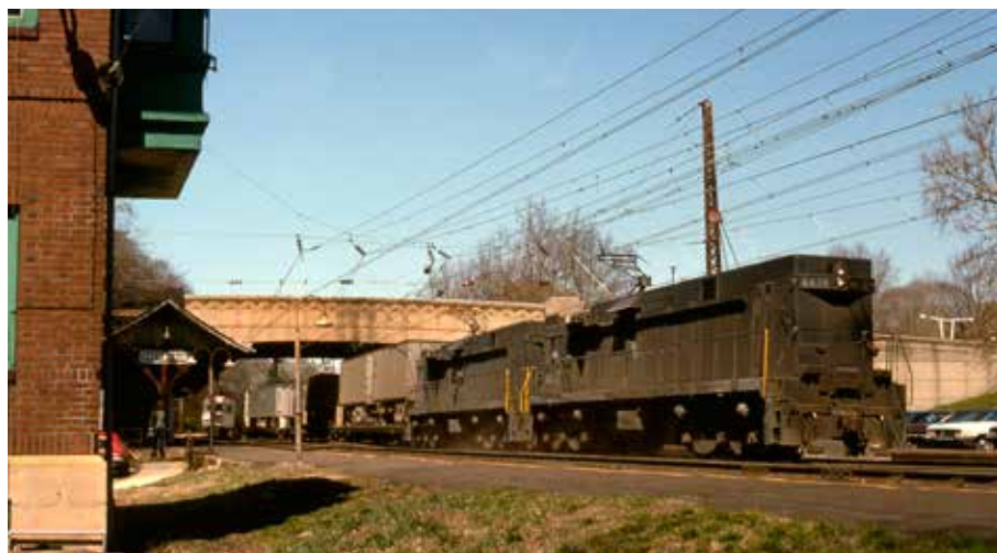
With Overbrook tower presiding at the left, grimy PC E44s 4418 and 4412 drift through the station with an eastbound piggyback train on April 8, 1975. The 66-unit E44 fleet, built by GE during 1960–63, was the backbone of PRR, PC, and Conrail electric freight operations.
