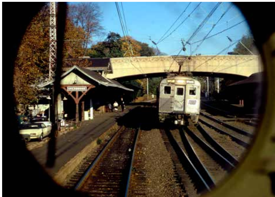
At Overbrook, a porthole window at the rear of an inbound MP54 train on Track 1 frames Penn Central Silverliners on Track 2 in 1970. By crossing under the City Avenue bridge, the trains have just entered Philadelphia. The circa 1860 depot has long been the Main Line’s oldest.
