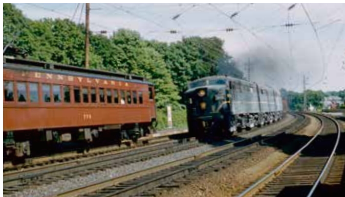
In the PRR era, MUs worked the locals, and electrics led nearly all through passenger trains, but steam and, later, diesels handled some freights. Westbound Alco FAs pass MP54s at Rosemont in June 1960.
