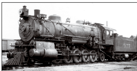
Santa Fe 2-10-2 No. 977 exhibits the tandem compound cylinders with which the 900s were built. R. P. Middlebrook, Stan Kistler collection
