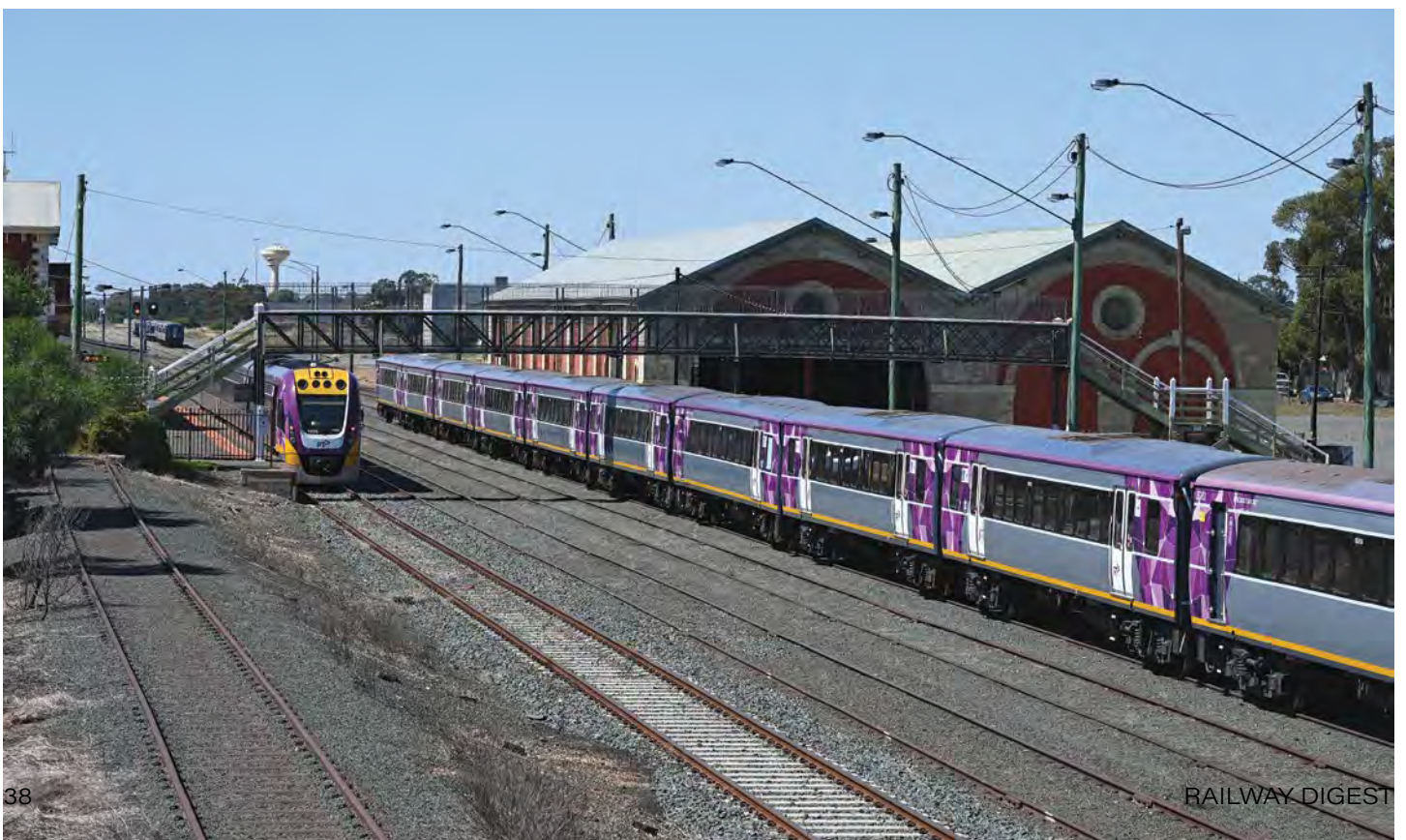
Below: Echuca yard appears quite deceptively busy in this view on Wednesday 20 December 2023. VLocity 35 at the station will shortly form the 11:15 service back to Melbourne. The four sets of "H" type carriages, each of six vehicles, seen in various places around the extensive yard are all stored, pending presumed disposal. These carriages started life from 1956 as suburban electric "Harris" (blue) trains, being converted to loco-hauled types in the 1980s. David Campbell
