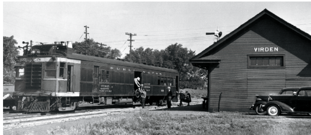
Gas-electric motor cars were the first successful applications of internal combustion on railroads. Chicago, Burlington & Quincy No. 9838, an Electro-Motive product built by St. Louis Car Co. in 1927, stops at Virden, Ill. It was powered by a 275-hp gasoline engine. Gordon Lloyd Sr.
