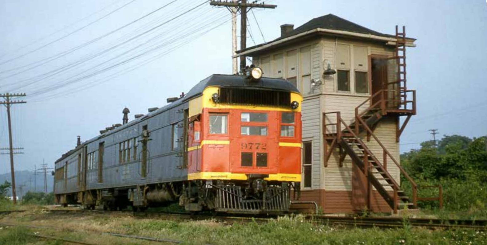
CB&Q motorcar 258 works as train 56 in Peoria, Ill., in June 1958. It has compartments for baggage, mail, and passengers and is towing a combine. Monty Powell, Denny Hamilton collection
