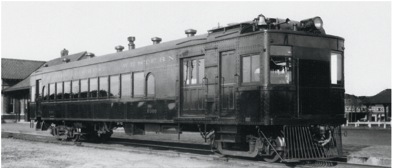
The beginning of it all: 150-hp Chicago Great Western gas-electric M-300, built in 1924, was the first railcar sold by Electro-Motive and founder H. L. Hamilton. The pioneering car was destroyed by fire. CLASSIC TRAINS collection
