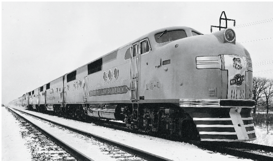
Union Pacific E2 No. LA-1, co-owned with Chicago & North Western, helped bring EMC out of the motorcar era. It sports the bulbous nose unique to that 1937 model. CLASSIC TRAINS collection
