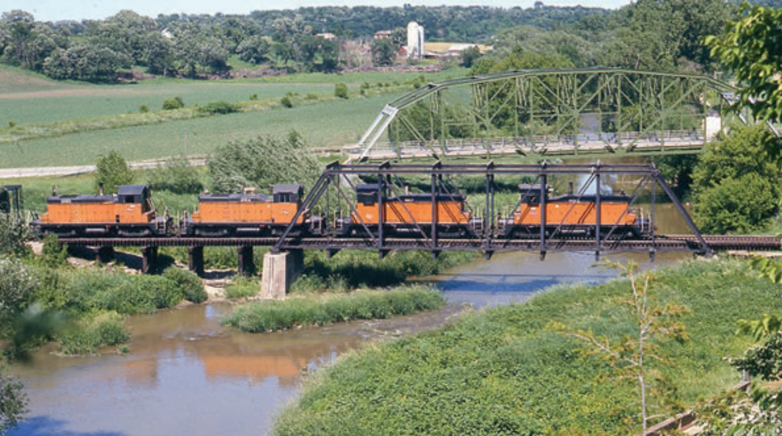
Milwaukee used SW1s in multiple on its 105-mile La Crescent–Austin secondary line along the Root River in southeast Minnesota; crews called them “Pups.” The line had weight-restricted track and bridges, exemplified here as an eastbound quartet makes a side trip on June 14, 1976, to Preston, base for the 50-mile Isinours–Caledonia branch. MILW’s 25 prewar SW1s came in the 1620 series, later were 900s, then 800s.
