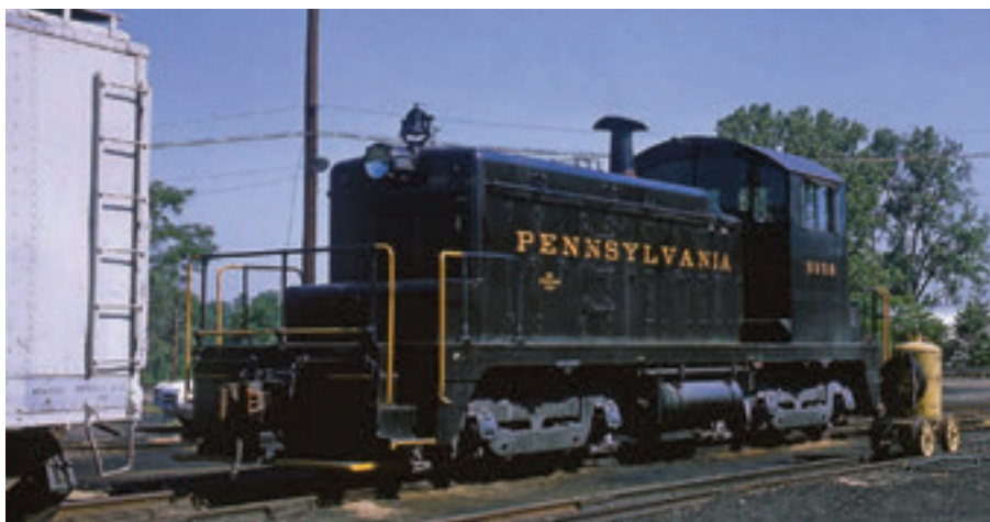
Pennsy's 85 SW1s, classed ES6, were the second-largest SW1 fleet, all but one (from 1942) built during 1946-50. PRR assigned some to remote, light-duty jobs such as with 5950 at Columbus, Ind., on June 3, 1964. Typical of Pennsy, the ES6s were in scattered number groups.
