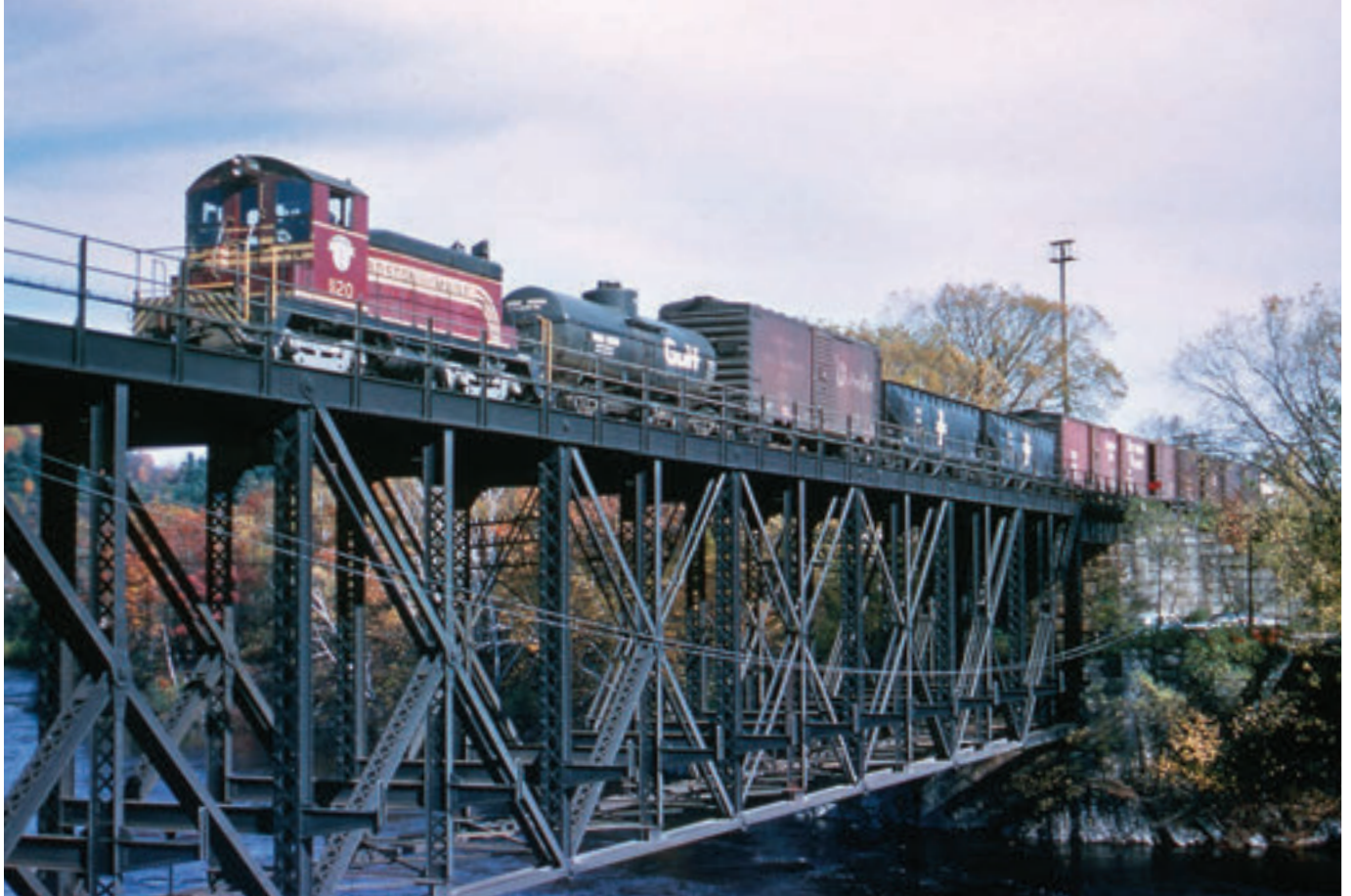
Boston & Maine dolled up its 14 postwar SW1s, intended for branchline service, in road colors, with big, angled engine-number boxes atop the front corners of the hood. No. 1120 crosses the Connecticut River bridge leaving Woodsville, N.H., for Wells River, Vt., in October 1962.
