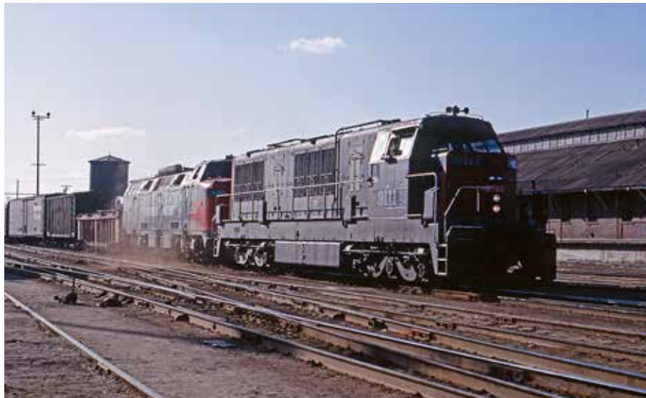
Dissatisfied with the relatively low-horsepower offerings of the domestic locomotive builders, SP acquired 21 4,000 h.p. diesel-hydraulic units built by Germany's Krauss-Maffei in 1961 and '63. K-M road-switcher 9111 leads cab unit 9104 at Bakersfield in October 1966.
