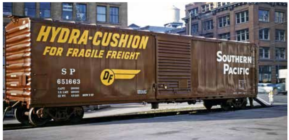
A leader on many fronts, SP under Russell developed the hydraulically cushioned freight-car underframe, a technology adopted throughout the rail industry. The first boxcar to wear SP's HYDRA-CUSHION paint scheme gleams on the downtown San Francisco team track in July 1957.
