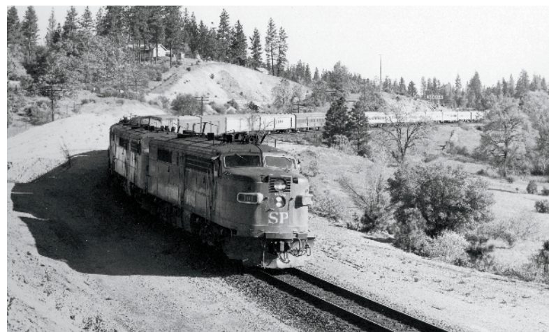
Alco PAs approach Auburn, Calif., as they descend the west side of Donner Pass with the City of San Francisco in 1967. SP's 64 units constituted the largest PA-PB fleet, nearly 22 percent of the total built.
