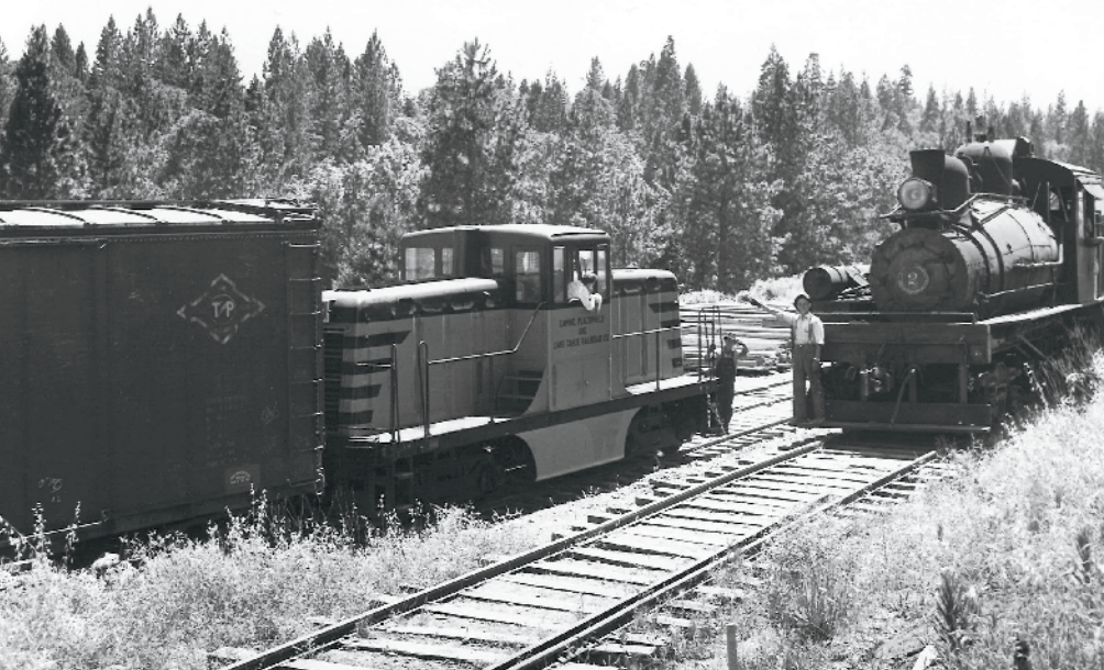
The victor meets the vanquished: GE 44-ton No. 101 works alongside Shay No. 2 in a November 1953 publicity photo. The railroad expected to cover the purchase cost of the diesel within six years, figured at a $12,000 savings each year. The single diesel unit replaced two steam locomotives by working faster, especially on the grades up to 5 percent, and eliminating the need for water stops. The railroad would later acquire a second 44-ton diesel from Burlington Northern. The steam locomotive is preserved at Travel Town Museum in Los Angeles' Griffith Park; regrettably, Shay No. 1 was scrapped after dieselization. CLASSIC TRAINS collection
