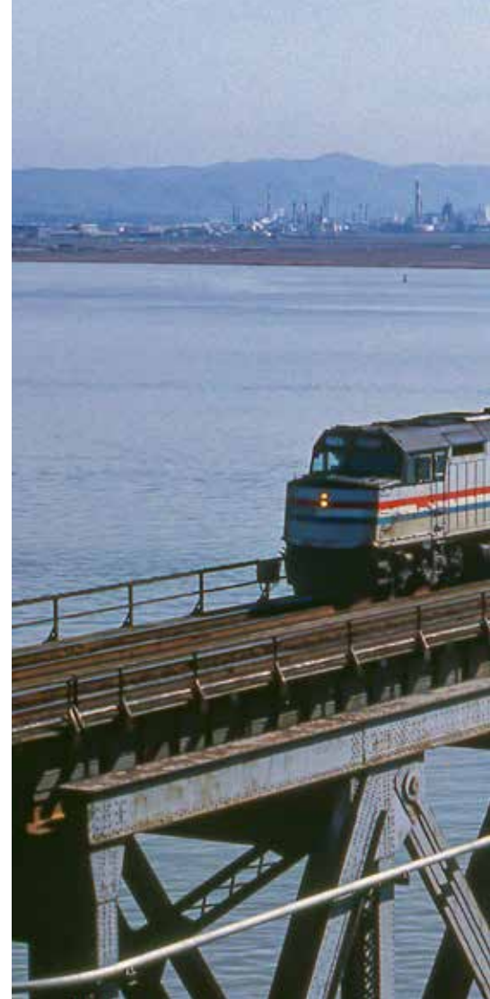
Amtrak's eastbound California Zephyr , led by a pair of F40PH locomotives followed by a Material Handling car and two heritage baggage cars, crosses Southern Pacific's 5,603-foot-long, vertical-lift bridge across the Carquinez Strait, adjacent to San Pablo Bay, on Feb. 16, 1990.
