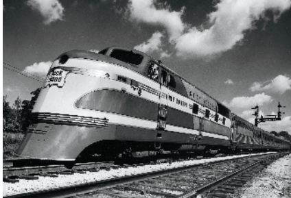
The Rock Island's TA diesels appear at first glance like early E units, but they are shorter and ride on four-wheel trucks. Rock Island
