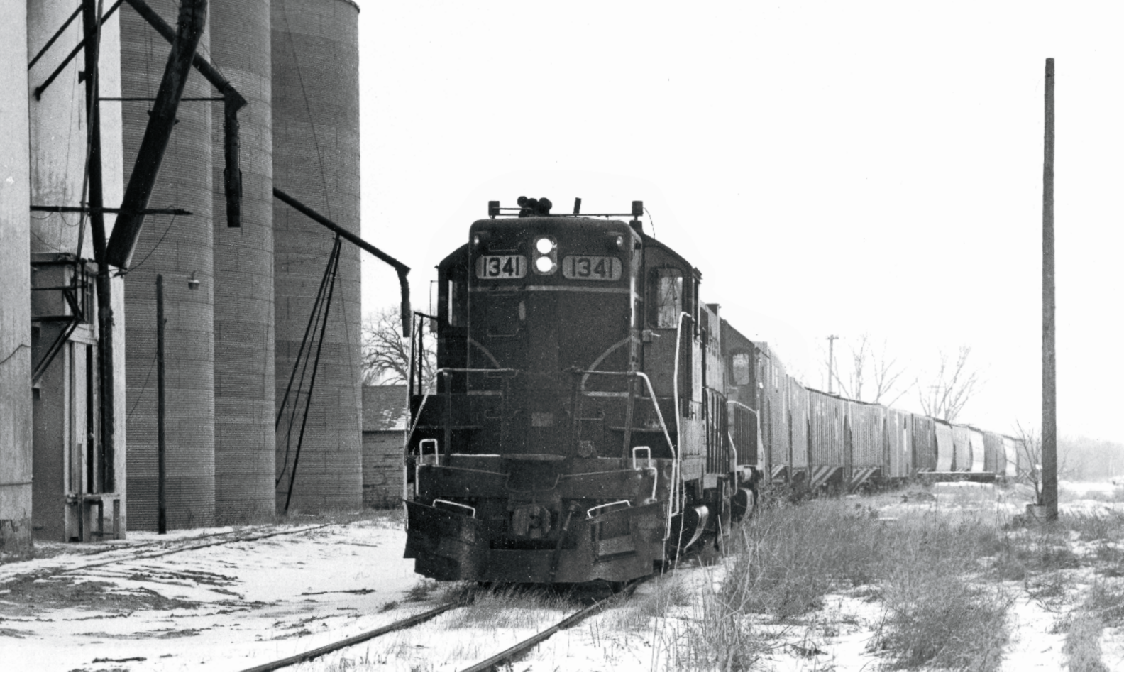
In January '80, train 340 works the Co-Op siding at Dows, Iowa. "I spent a lot of time on the 1341," Lasher recalls. "The GP18s were good engines, but had one flaw. With the throttle in notch 2 . . . everything in the cab would join in an aggravating cacophony of sympathetic vibration."
