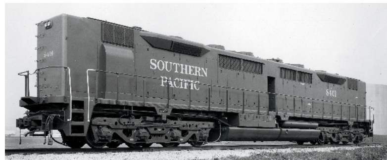
SP 8401 shows the DD35's square ends and four-axle trucks. All EMD DD models had a passageway between the engine compartments.
