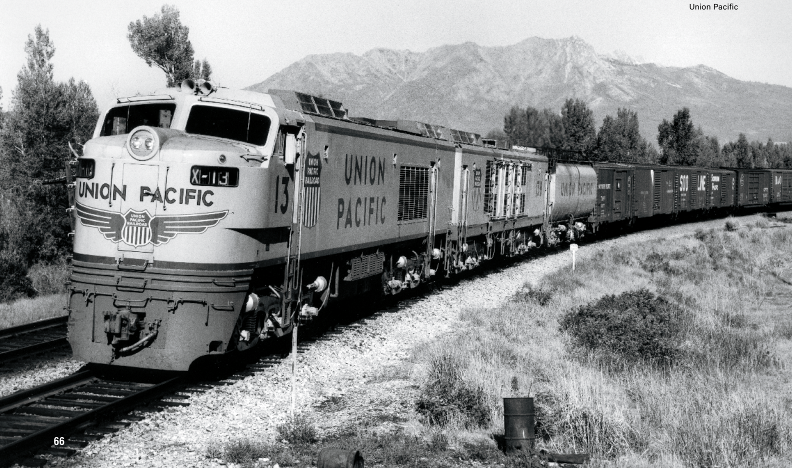
This undated public-relations photo showcases UP 8,500 h.p. turbine No. 13. The A unit housed auxiliaries; the turbine was in the B unit.
