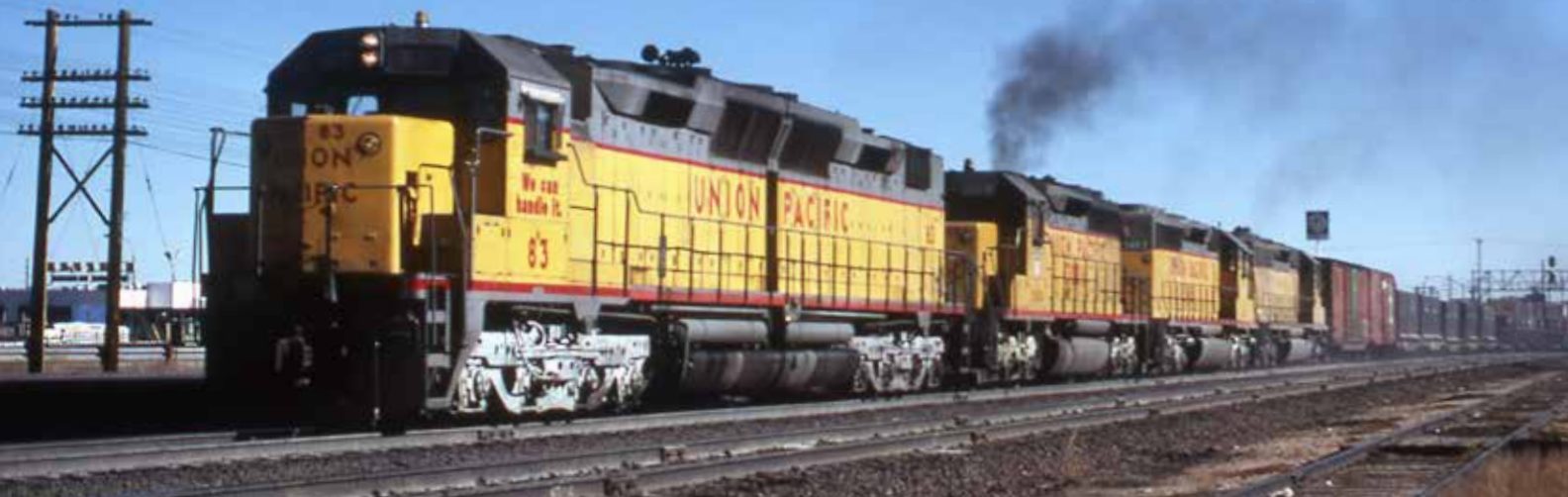
UP DD35A No. 83 leads a westbound train out of Cheyenne, Wyo., in October 1978 with three SD40-2s producing a total of 14,000 horsepower.
