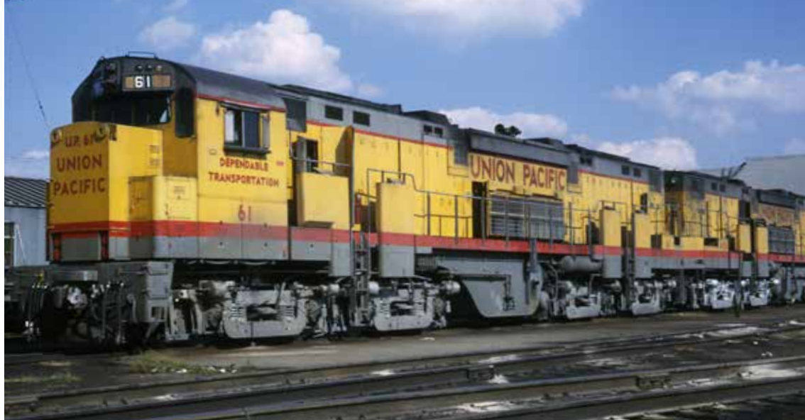
Alco C855 No. 61 rests at the diesel pad at Council Bluffs, Iowa, in September 1966 with a mate. When run as intended in a three-unit set, they produced 16,500 h.p., more than any other double-diesel offering.
