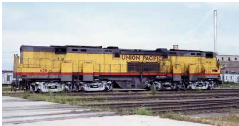
The sole C855B unit, No. 60B, rests at Council Bluffs between runs in July 1967. Four sand boxes hang from the frame outside the handrails.
