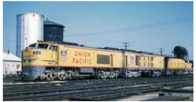
Turbine No. 1 rests at Council Bluffs in September 1960. The giant locomotive, including tender, stretched 179 feet and weighed 592 tons.
