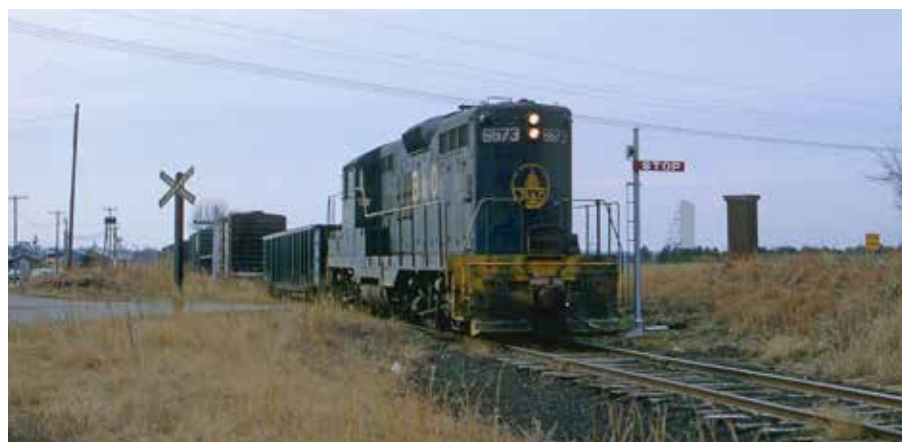
Having stopped for the Arenzville Road crossing, GP9 6673, a former C&O unit, leaves Beardstown on March 11, 1970, for Springfield. B&O's Geeps were set up long-hood-forward, C&O's the opposite, but by this time, B&O's Beardstown wye connection to CB&Q was long gone.
