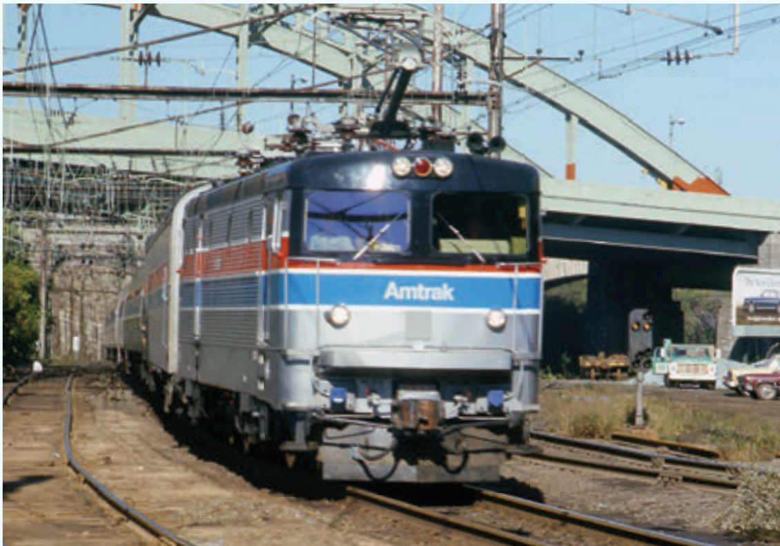
Swedish Rc-4a demonstrator X995, on loan for testing and shown southbound at Baltimore in October 1976, was the precursor of the successful fleet of AEM7 electrics built by Swedish firm ASEA and America's EMD.
