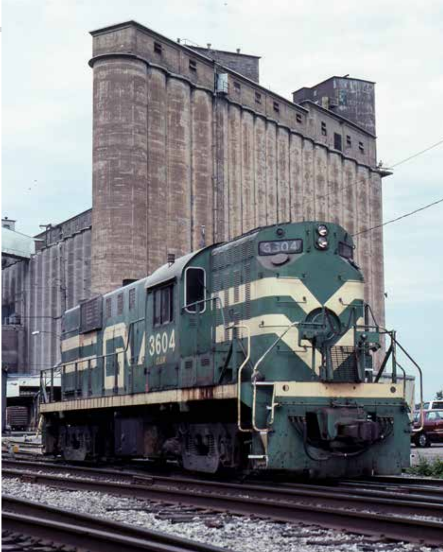
Empire builder: one of two former Central Vermont RS11s that helped Genesee Valley Transportation get its start, DL&W 3604 holds down a contract switching assignment at Buffalo, N.Y.
