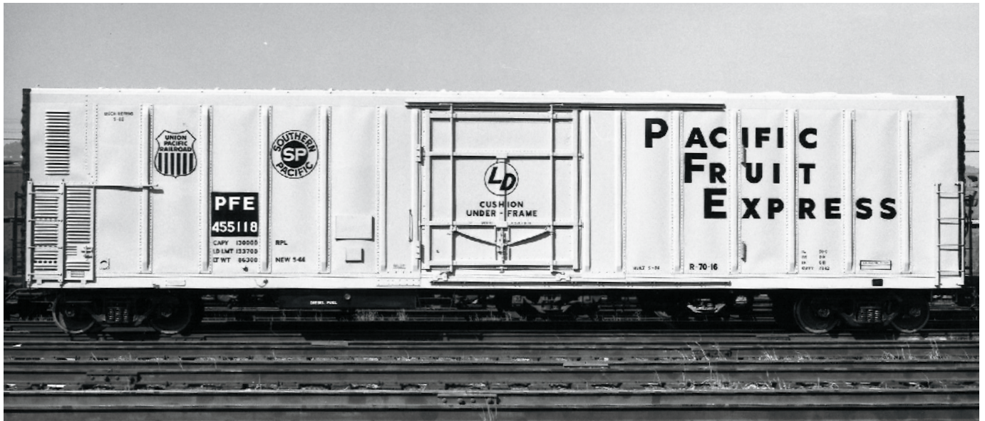
Pacific Fruit Express 57-foot mechanical reefer No. 455118 is exemplary of hundreds of such cars in use in the early 1970s to move West Coast produce to Midwest and Eastern markets. PFE was a joint venture of Southern Pacific and Union Pacific. Classic Trains collection
