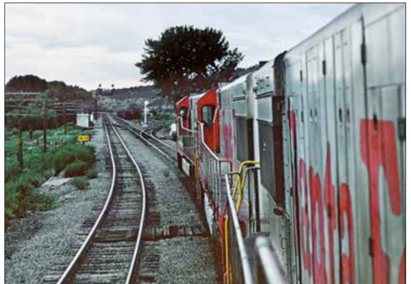
Test Run 3 is just out of Trinidad, Colo., as it hits the base of Raton Pass, whose 30-mph passenger limit was more than the train could manage. Nightfall precluded any photos west of here. Grades and wind helped nix this route for the Super C .
