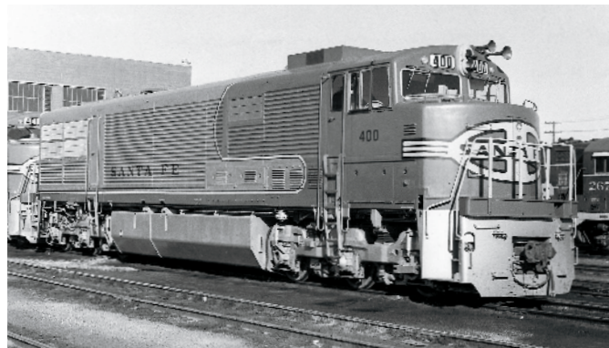
No. 400 marks its first day on Santa Fe property at Kansas City in November 1967. The U30CG was the only General Electric passenger U-boat model with a full cowl body. Jerry F. Porter
