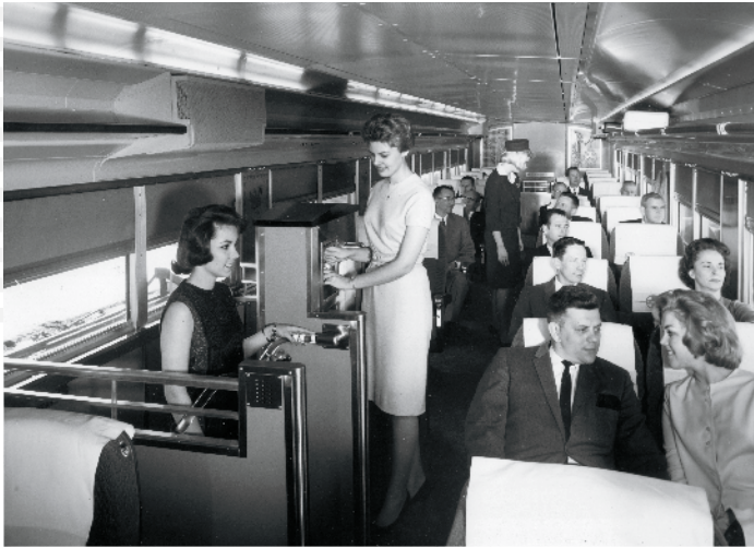
After boarding Hi-Level coaches, passengers climbed stairs to the main seating area (above left), where end doors provided car-to-car access (above right). Luggage shelves were below (right).
