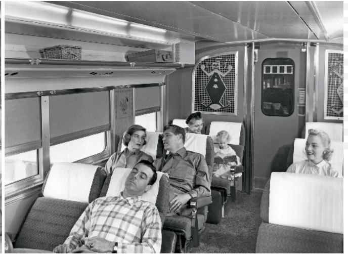
After boarding Hi-Level coaches, passengers climbed stairs to the main seating area (above left), where end doors provided car-to-car access (above right). Luggage shelves were below (right).
