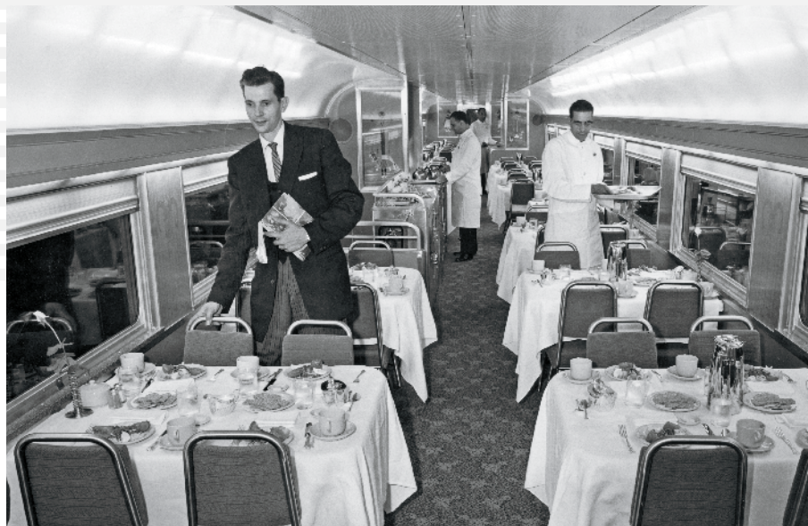
The 96.7-ton Hi-Level diner required six-wheel trucks. Each car sat 80, at 19 tables for 4 plus two pairs. The 36-foot, all-electric kitchen was below, with a dumbwaiter to move the food.
