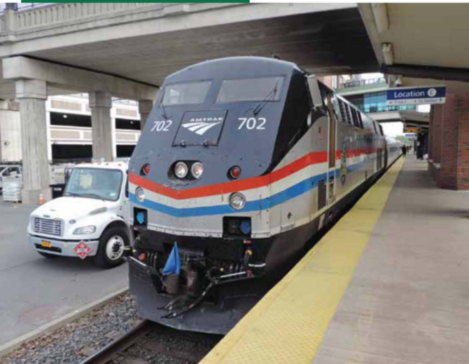
ABOVE With a blue flag tucked into the coupler, P32AC-DM 702 is fueled on Track 3 at Amtrak's Albany-Rensselaer, N.Y., station. SCOTT ORNSTEIN
