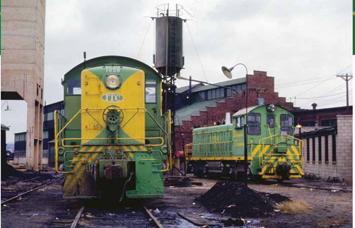
Alco and EMD units repose at the Illinois Terminal's Federal Yard at Alton, Ill., in March 1970. Note the Flexicoil truck on the SW1200 at right.
