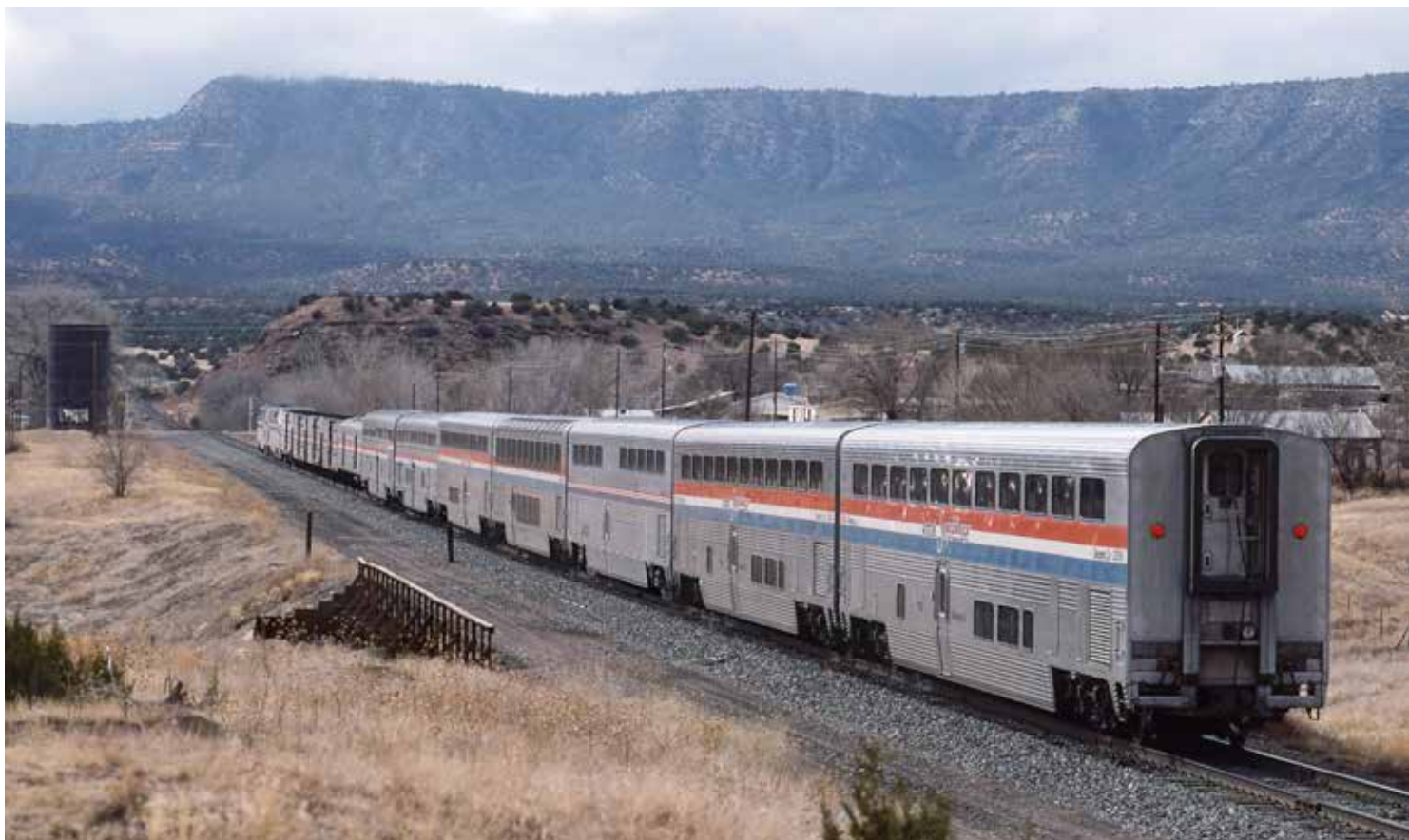
The Santa Fe Hi-Level cars were the template for Amtrak’s Superliners, introduced in 1979. In this March 1995 photo of the westbound Southwest Chief at Ribera, N.Mex., the last five cars are Superliners, while the two ahead of them are ex-Santa Fe Hi-Level coaches. John C. Lucas
