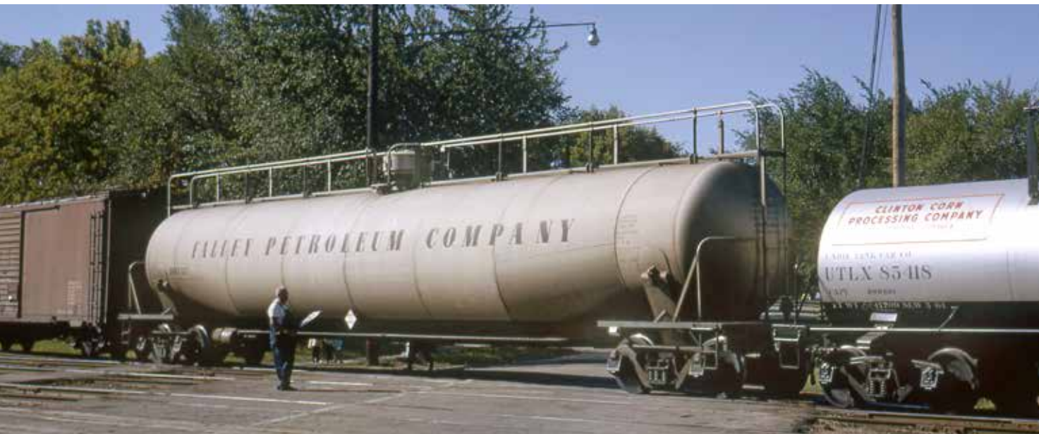
Large tank cars became common in the 1960s, especially for light-density products such as liquefied petroleum gas. General American built this 100-ton, 30,200-gallon car in 1962. Multi-diameter tanks like this one were built through the late 1960s. John S. Ingles
