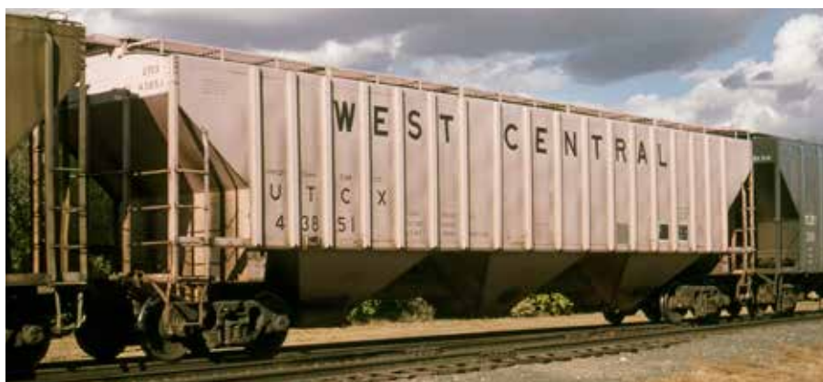
Pullman-Standard's 4,750-cubic-foot PS-2 covered hopper was the most popular grain car of the 100-ton era, with more than 56,000 built from 1966 to 1972. This car, part of Union Tank Car's lease fleet, was built in 1980. Scott E. Russell, Brian Schmidt collection
