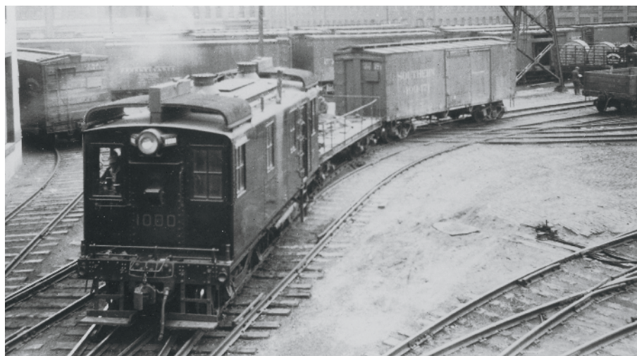
Jersey Central No. 1000, the 1925 Alco-GE-IR box-cab hailed as the first commercially successful diesel-electric, switches at the road's Bronx freight terminal. Frank DiFalco collection
