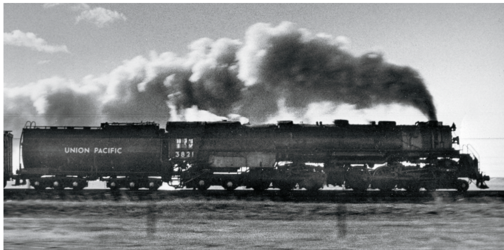
Alco and Union Pacific jointly designed the first 4-6-6-4s in 1936. The builder supplied the road with 105 Challengers through 1943; No. 3821 was built in 1937. Robert Hale
