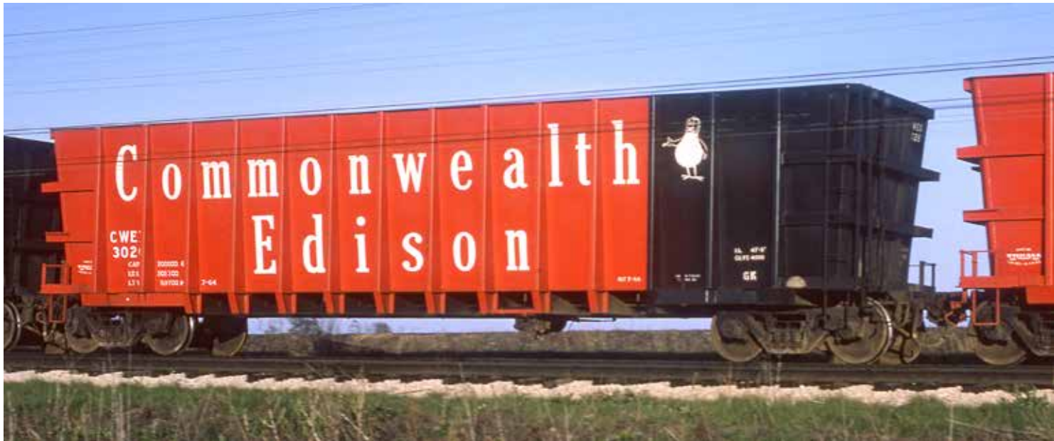
ComEd's Thrall-built 100-ton, 4,000-cubic-foot coal gondolas, built in July 1964, were the first unit-train cars equipped with rotary couplers (on the black end). This enabled them to be unloaded without uncoupling. Thrall built versions of this car through the 1970s. J. David Ingles
