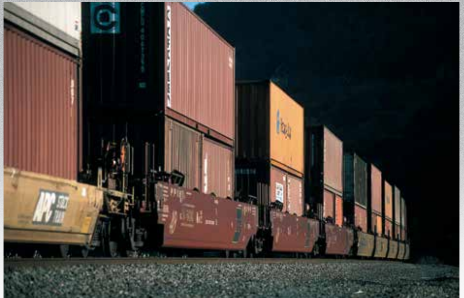
Intermodal took a great leap upward with the double-stacking of containers in the early '80s. First employed for import traffic, the concept spread to domestic freight. Matt Van Hatten
