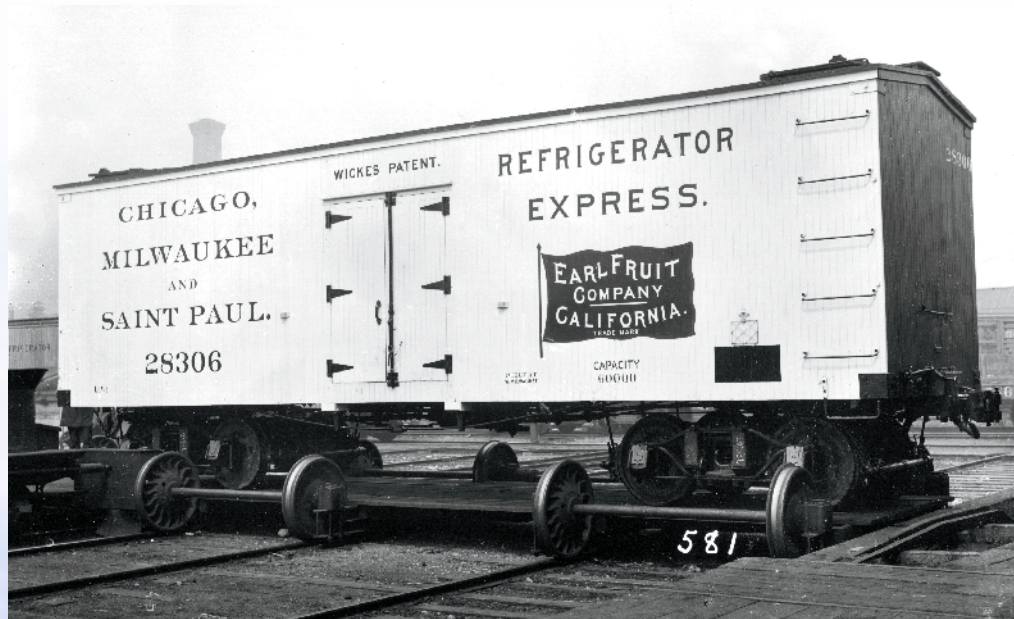
This 32-foot, 30-ton capacity ice-bunker refrigerator car, built around 1900, features all-wood construction with a truss-rod underframe. CLASSIC TRAINS collection
