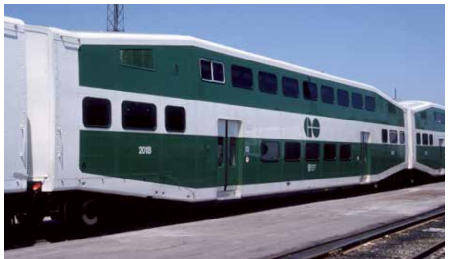
Hawker Siddeley, which acquired Canadian Car & Foundry in 1957, supplied lozenge-shaped cars to Toronto’s GO Transit in 1977. Their three-level format has since found wide use. Jim Hediger
