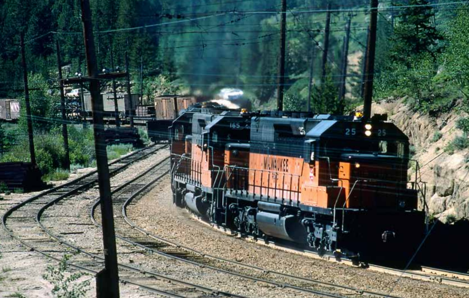
Milwaukee trains through Butte, Mont., were few by 1975, but we did chase this DFW—Dead Freight West—across Pipestone Pass. Led by SD40-2 No. 25, it is at Donald, atop the pass, running along a slide-detector fence at 15 mph. Poles and wires remain from the line's electrification, recently de-energized.
