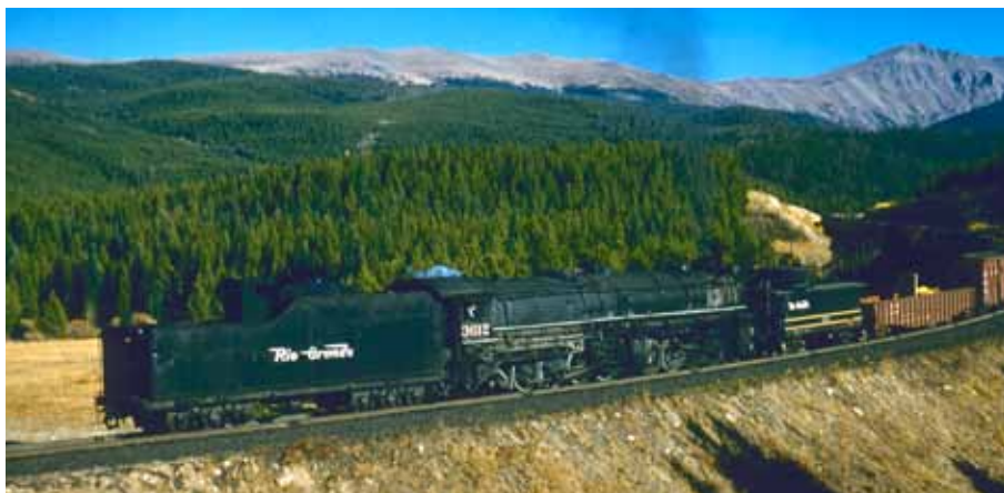
No. 3612, from D&RGW's last group of 2-8-8-2s (Alco, 1927), pushes near Winter Park in October 1956, deep twilight for Grande standard-gauge steam. The black caboose is typical.
