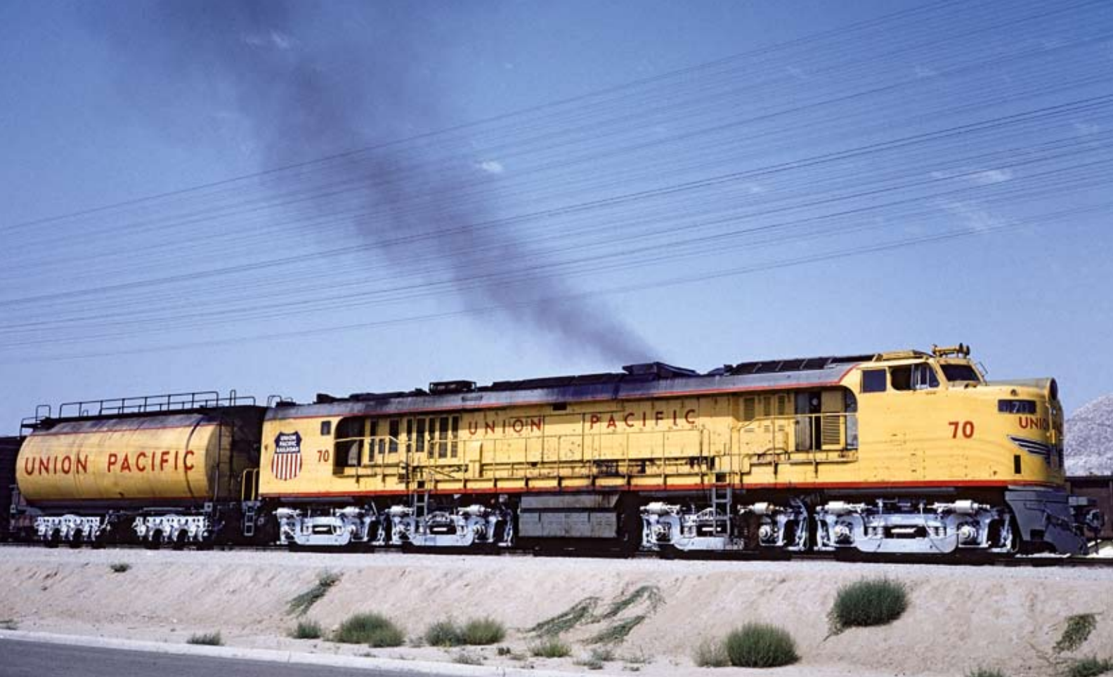
“Veranda”- or “gallery”-style turbine 70, a 4,500-h.p. model, shows off the “road-switcher” type carbody at Colton Tower, Calif., on July 28, 1962, as it prepares to head for San Bernardino and Cajon Pass.
