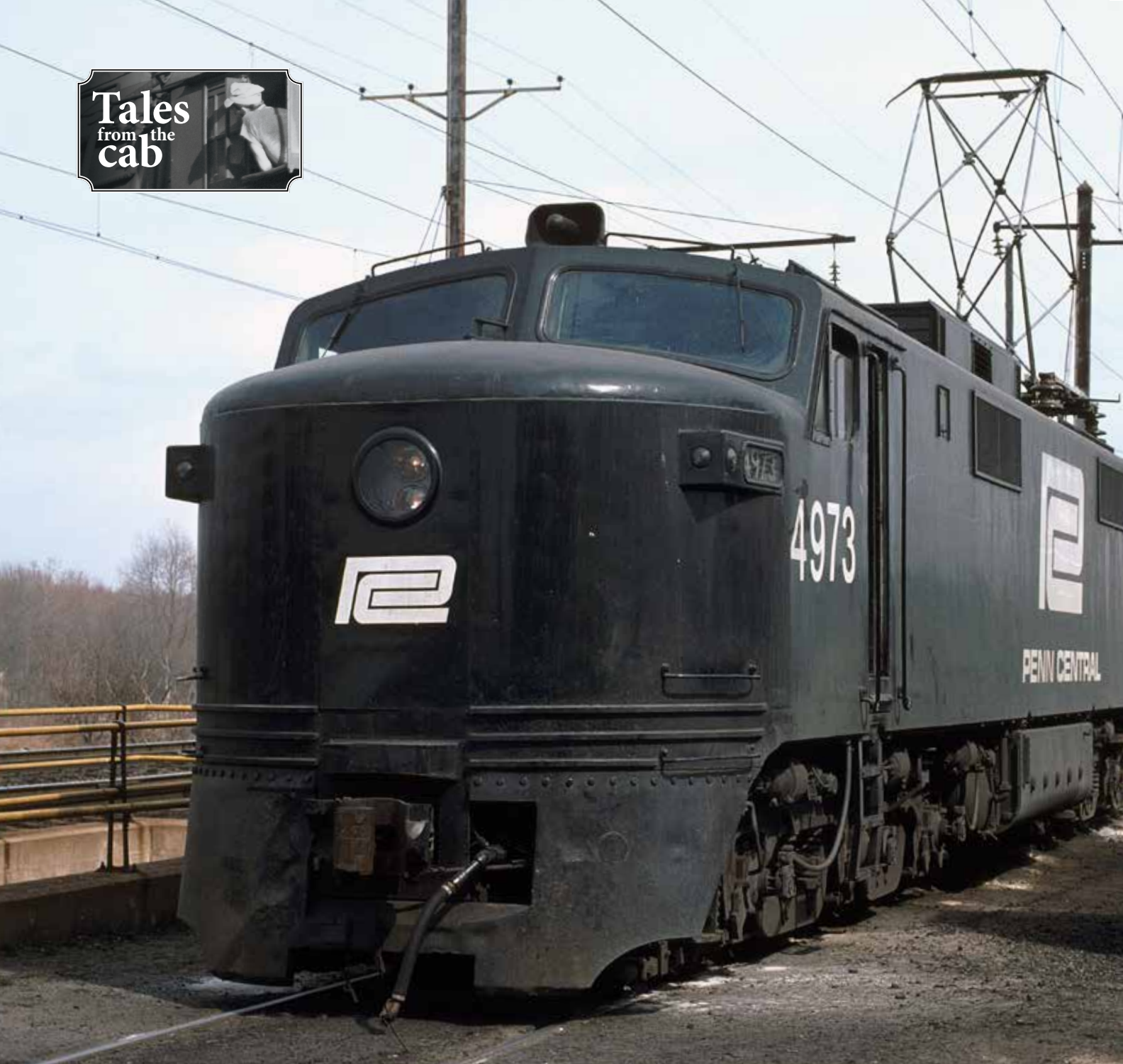
Author Jack Neiss's nemesis—Penn Central E40 No. 4973—stands at Morrisville, Pa., on March 21, 1976. Behind the former New Haven passenger motor are ex-PRR E44 freight units. Neiss liked the 4973's Hancock air whistle, but its exposed air-brake pipe caused him grief.
