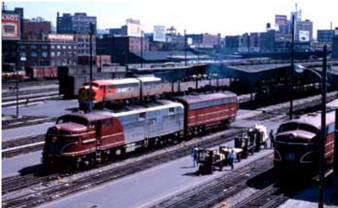
RI's sole surviving E3A, 1939-built No. 625 as one of two, idles with an F7B (from one of three passenger A-B sets) at Union Station July 21, 1962, after arriving on train 15. At right, RI's highest-numbered FP7, No. 411, awaits departure with train 39. Beyond the RI trains is what is likely Santa Fe's overnight Kansas City Chief from Chicago.
