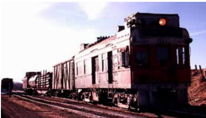
Early on April 7, 1962, the 9006 is ready to leave Horton with mixed 79 on its 6½-hour run to Fairbury. After RI's Horton Shops in 1927 installed two 275 h.p. 6-cylinder distillate engines in a pair of 1911-built 40-foot mail cars, the road in 1929 took three baggage cars, put in twin 400 h.p. EMC power plants, and numbered them 9005–9007. Both the 9006 and 9014 last operated on this line in fall 1962.
