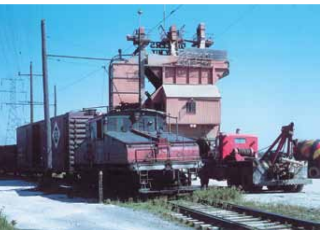
Motor 456 (left), one of a pair set up to work from overhead trolley or battery power, switches an industrial spur near Briergate. Three of NSL's four steeple-cab "pups" roll coal hoppers south at Deerpath in June 1951. Two 8-axle motors rounded out the road's 1950s locomotive roster.
