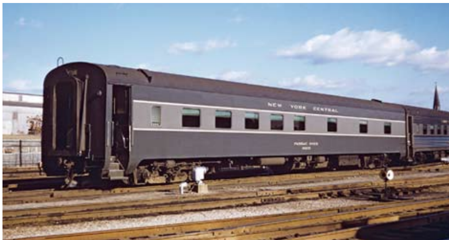
Typical of NYC sleepers which lost their "Pullman" identification was 10235 Passaic River (at Detroit in 1961), among 97 River 10&6's in lot 6790 delivered by Pullman-Standard in 1948-49.
