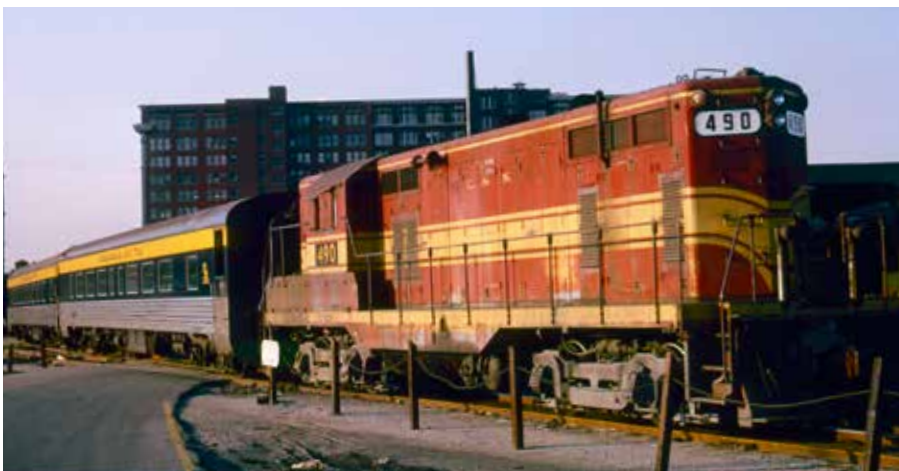
Among L&N switchers busy on Derby Day 1966 is GP7 No. 490, ex-Nashville, Chattanooga & St. Louis 700, built in 1950 and riding on Type B trucks, and not repainted nine years after merger.
