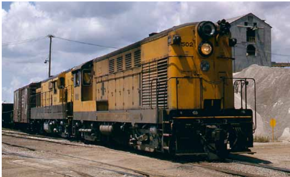
Two of Akron, Canton & Youngstown’s 15 bought-new Fairbanks-Morse units, H20-44 502 and 208, its last H16-44, switch at Carey, Ohio, on July 28, 1963. Check out the 502’s horns!
