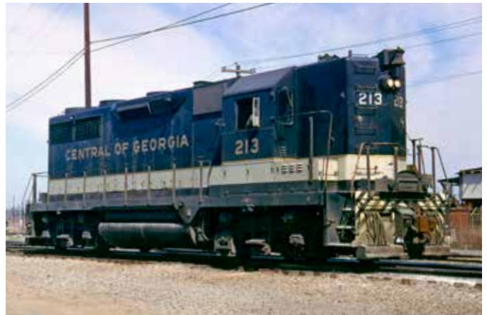
Central's penultimate group of new diesels was five GP35's, 210–214, delivered in December 1963. The 213 posed at Augusta in March 1966.
