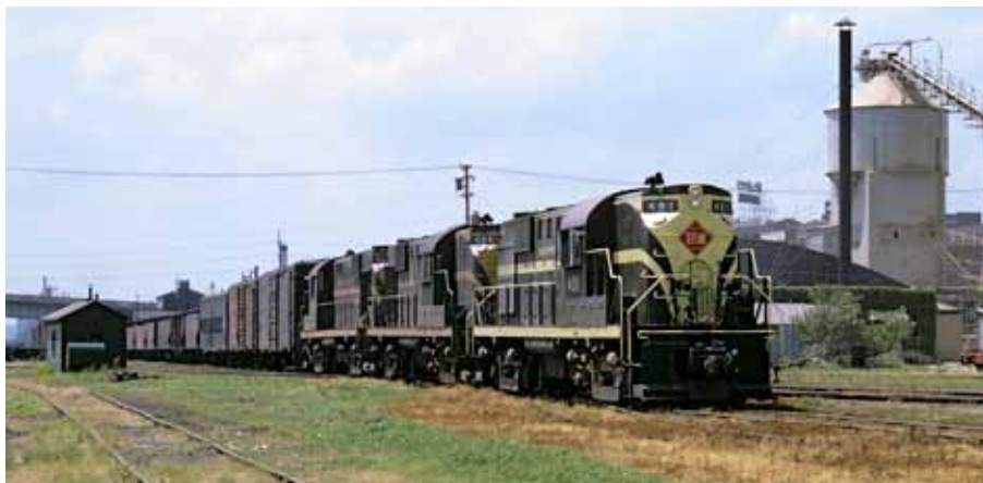
All three of TP&W's RS11's, built 1958-59, enter Peoria from the west in June 1963. Lead unit 401, with the "newer yellow" trim, would eventually get chop-nosed. Sister 400 is preserved.
