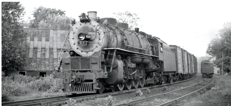
Rutland's L-1 4-8-2s, Nos. 90–93, were pretty but short-lived, built in 1946 but cut up in 1955 to pay for new diesels. In August '52, No. 93 rolls through Proctorsville on one of her last trips.
