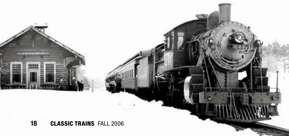
Ancient 1904 Cooke 2-6-0 No. 33 leaves Rome, N.Y., in 1936 under a canopy of steam.
