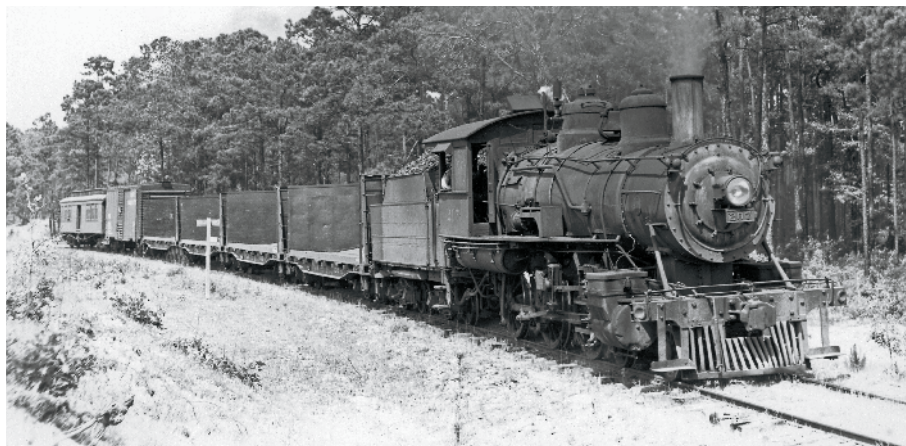
More typical of the steam-era G&F than a “mainline” doubleheader was this branchline mixed behind 4-6-0 No. 207 at Garfield, Ga., on May 12, 1950. Note the partitioned coach at the rear.
