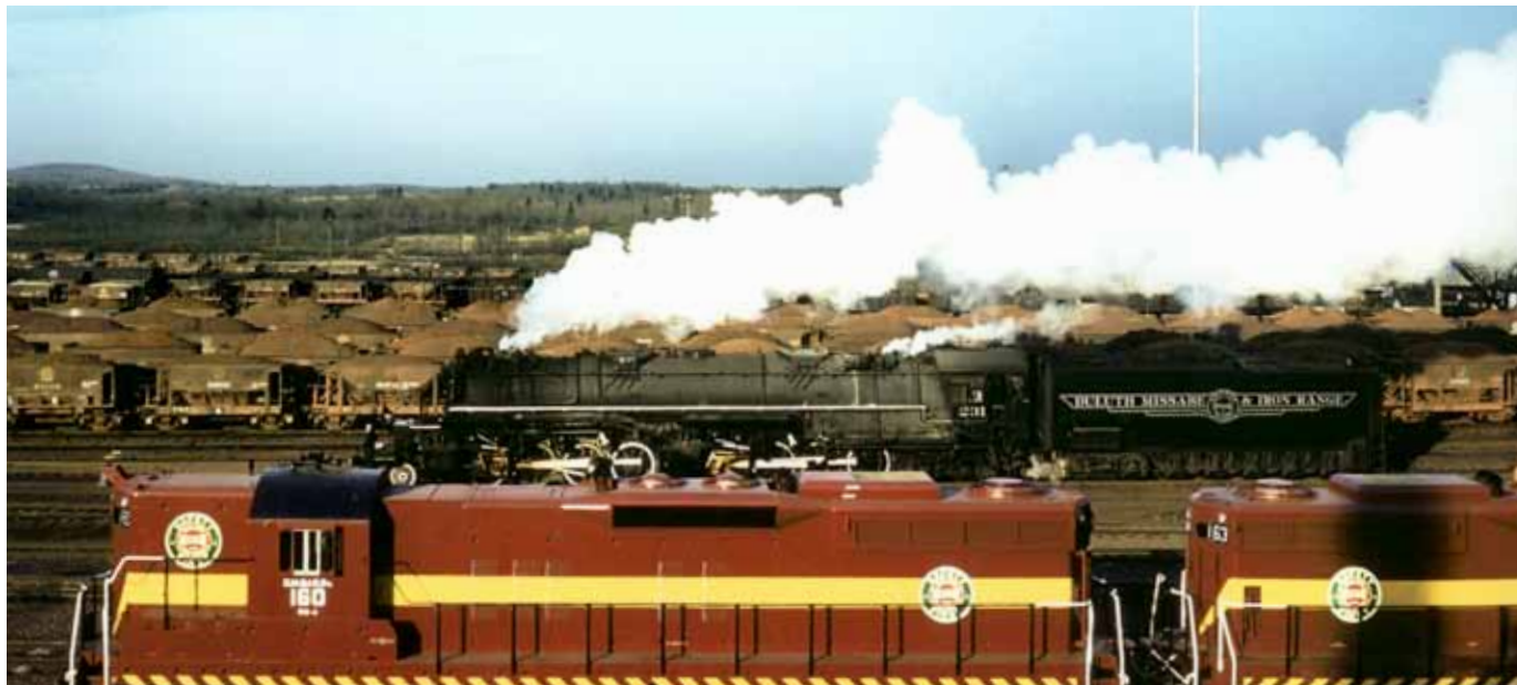
No. 231, one of Missabe's 18 famous Yellowstone 2-8-8-4s, passes two brand-new successor SD9's (among 74) at Proctor Yard in May 1959.
