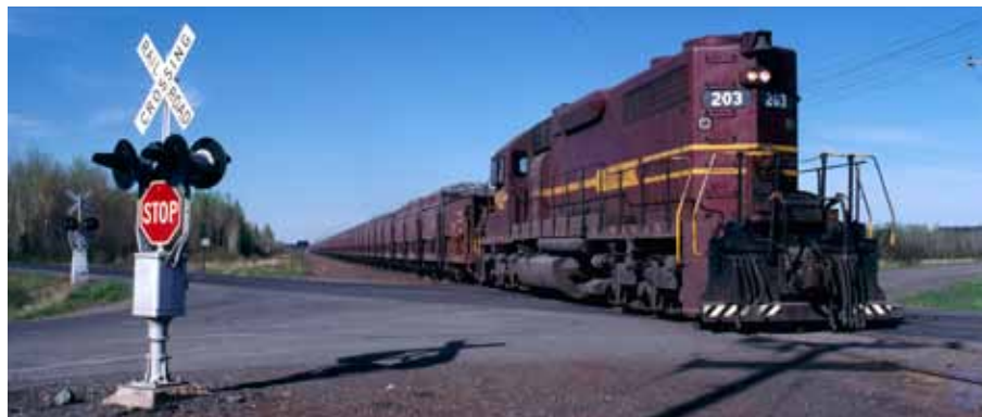
SD38AC No. 203 splits a Route 7 intersection near Virginia with a May 27, 1979, Thunderbird Mine raw-taconite shuttle to Fairlane. The SD38's had bells on the long hood for the shuttles.
