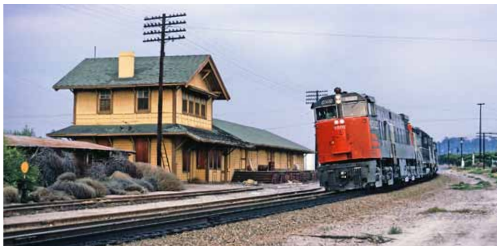
U50 No. 8502 curves past Bryn Mawr with a westbound freight on March 28, 1965. GE built 26 of the distinctive diesels (3 for SP, 23 for UP) in 1963–65; wheel arrangement was B-B+B-B.
