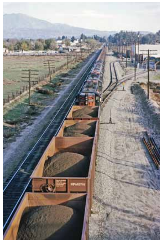
U50 No. 8502 curves past Bryn Mawr with a westbound freight on March 28, 1965. GE built 26 of the distinctive diesels (3 for SP, 23 for UP) in 1963–65; wheel arrangement was B-B+B-B.
