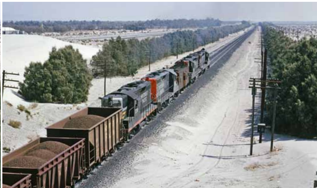
At Thousand Palms, start of the steepest part of Beaumont Hill, a lucky 13 units—11 SD9's and 2 GP9's—roar west with Kaiser ore in September 1965. Unusually, there are two sets of power on the rear bracketing the caboose, not the customary one ahead of it.
