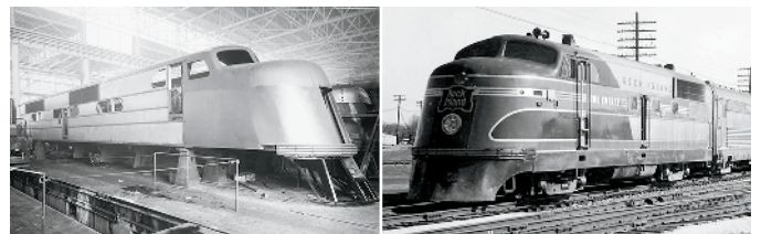
EMC's planned standard line of similarly styled passenger diesels consisted of the twin-engined EA (left) and the single-engined TA.
