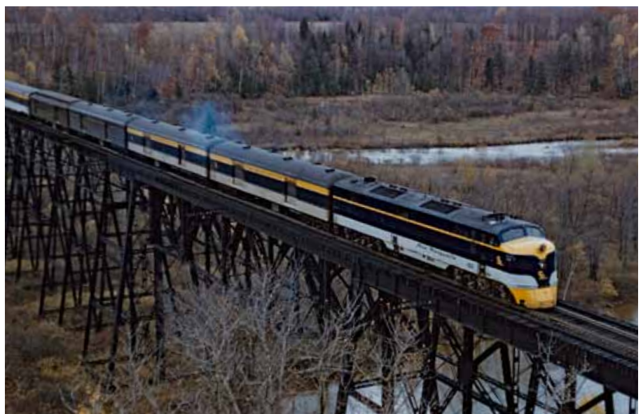
E7 102, one of eight Pere Marquette E7's ordered before its June '47 merger into C&O, leads Grand Rapids–Petoskey, Mich., train 105 across the 1,170-foot-long High Bridge, 98 feet above the Manistee River 5 miles north of Wellston. C&O removed the bridge in 1955. John B. Corns coll.
