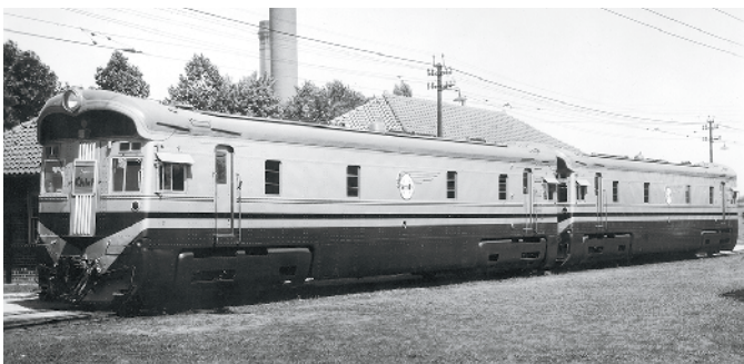
The final two twin-engined box-cabs, Santa Fe's "One-Spot Twins," with special livery and roof cowling, worked the original Super Chief .
