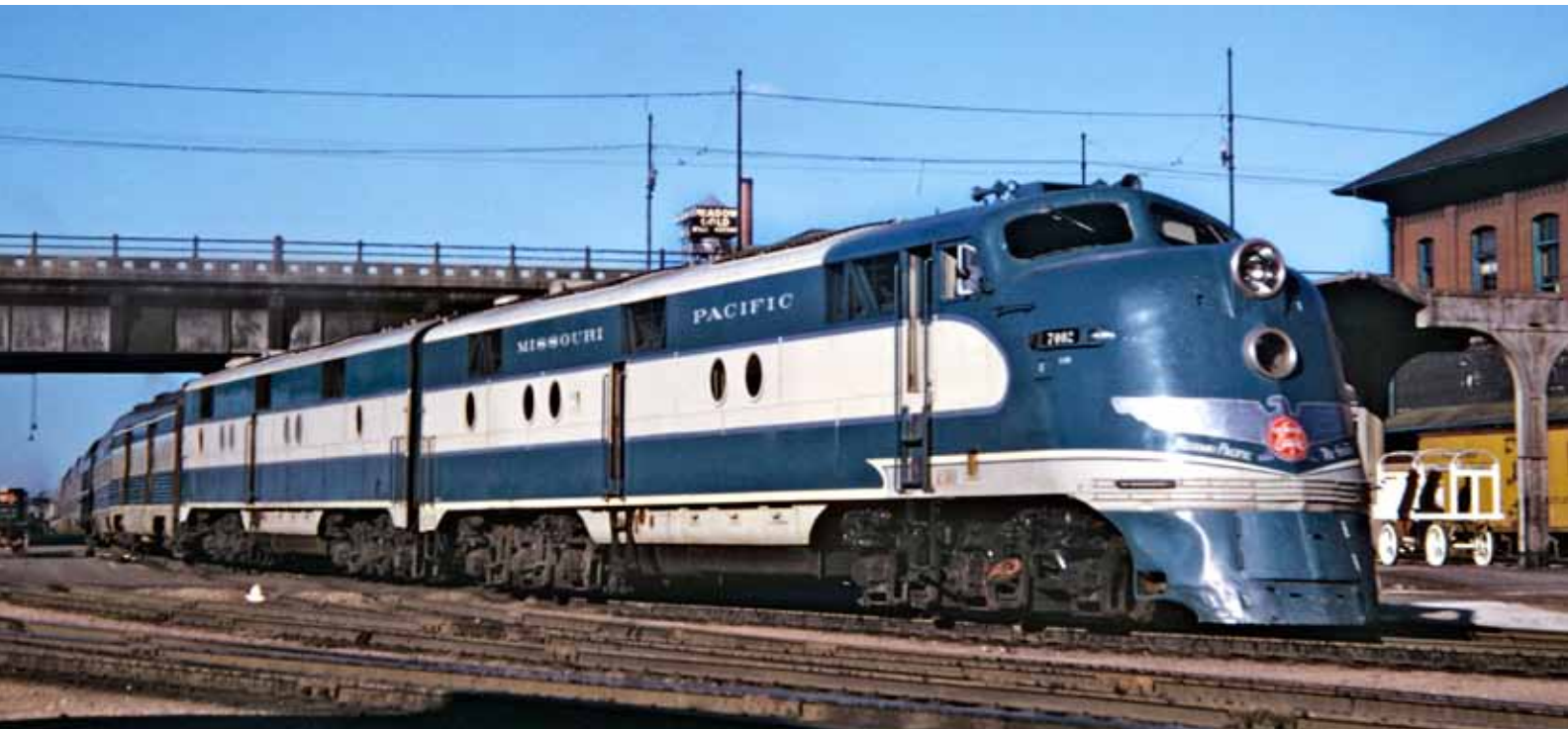
MoPac 7002 and an E6B depart Denver with the Colorado Eagle in August 1947. The A unit carries the names of the train's two partners, MP and Rio Grande, below its eagle emblem. Most roads specified standard rectangular side windows, not portholes. Frank and Todd Novak coll.
