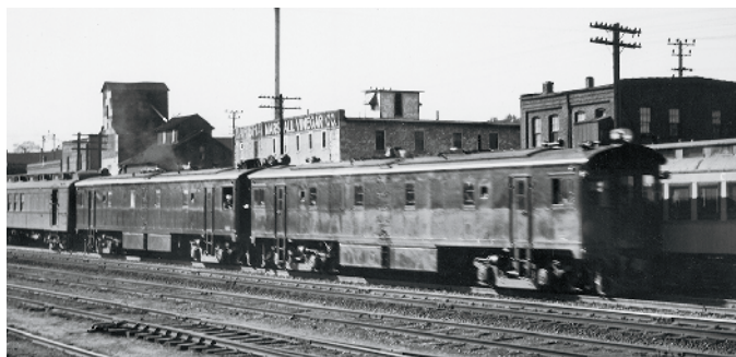
They weren't much to look at, but EMC 511-512 (on C&NW at Marshalltown, Iowa) proved the twin-engine concept that was the basis of the E.
