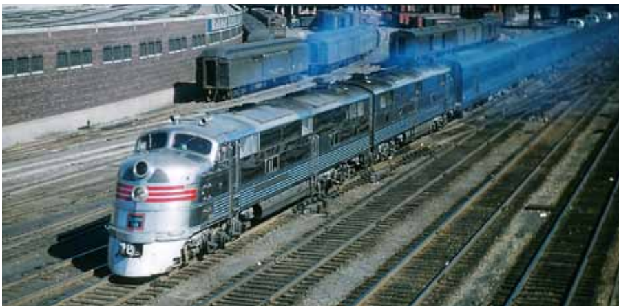
Still gleaming after nearly two decades, CB&Q 9912-A and another E5A accelerate the Morning Zephyr out of Chicago in 1958, after red nose stripes replaced black ones. Dan Pope coll.
