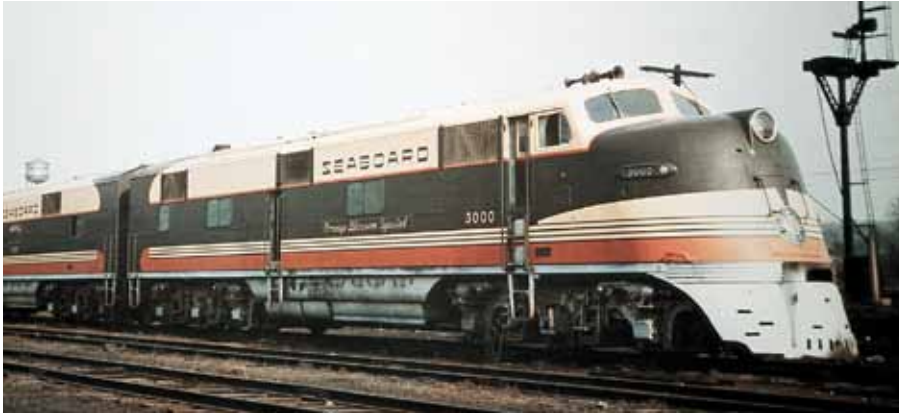
Seaboard 3000, at Washington in 1940, was the first E unit with Electro-Motive's 567 engine and electricals, a status EMD marked at its 1964 scrapping. O. H. Borsum photo, Paul Lubliner coll.
