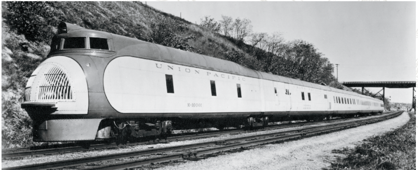
Unlike his M-10000 design, Blomberg placed the engine of UP M-10001 in a cradle between the trucks, as shown in his Patent 2,079,748, awarded after he left Pullman for EMC. Left, U.S. Patent & Trademark Office; above, Union Pacific
