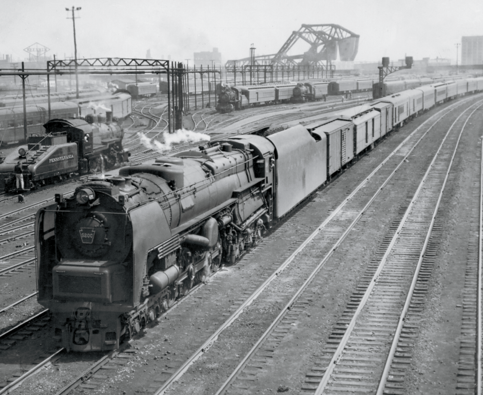
PRR 6200 brings the Manhattan Limited into Chicago on June 13, 1947; the S2 sports its second, larger set of smoke lifters. Working the coachyard are three B6sb 0-6-0's, sisters to the last active PRR steamer [see page 72].
