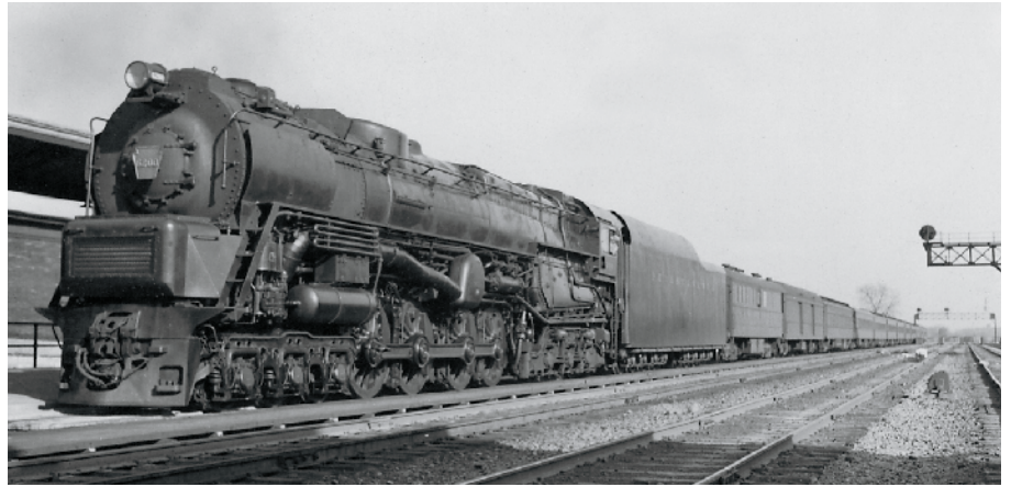
Turbine 6200, a test car tucked behind its tender, stops at Englewood, Ill., with PRR's New York-Chicago Golden Arrow. The small, curved smoke deflectors were an early addition.
