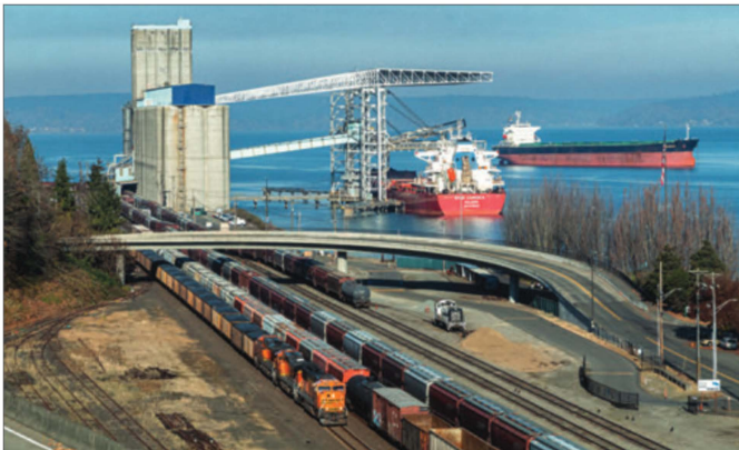
RIGHT: Uncommon SD70MACe BNSF 9749 leads a loaded coal train destined for Canada past the former NP Moon Yard in Tacoma on November 19, 2022. The TEMCO grain elevator uses part of this former NP yard for unloading inbound grain trains from both BNSF and Union Pacific.
