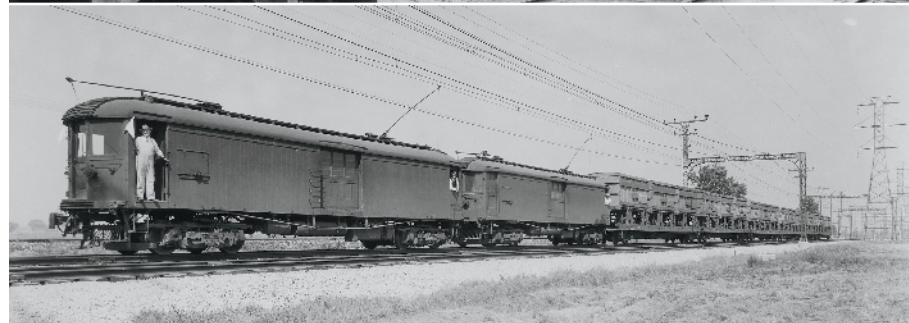
Top: North Shore box motors are loaded with LCL freight at the Montrose freight house in Chicago in 1927; heavy, hinged doors on the car at left identify it as one of the road's four refrigerated trailers. Above: Twin box motors head up a "ferry truck" piggyback train in 1928.
