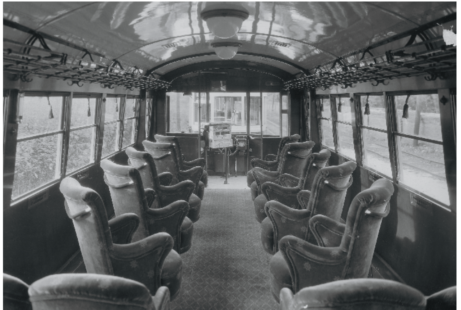
The wall contours of the curved-sides are apparent in this view inside the deluxe parlor car Cincinnati, built in 1926 for exhibit at a trade show. It became I&SE parlor 250 in 1929.
