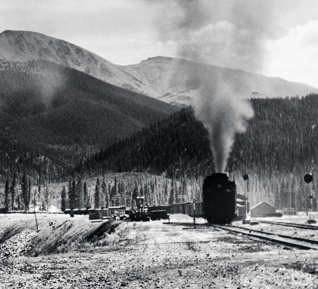
Business as usual: An eastbound Denver & Salt Lake freight enters Moffat Tunnel with 2-6-6-0s fore and aft. The Denver & Rio Grande Western absorbed the "Moffat Road" in 1947.
