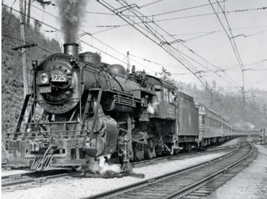
After unloading at Seattle Union Station, the Olympian Hi was towed south behind steam, backward and with diesels still attached, to a wye, where the train was turned to head for its ultimate destination, Tacoma. Eastbound, the process was reversed. Stuart B. Hertz
