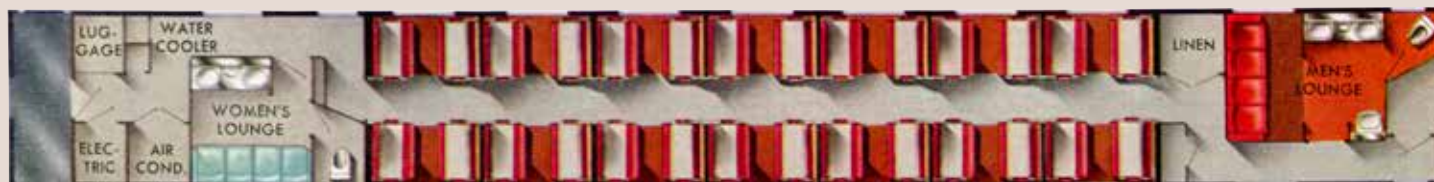
The Touralux cars had 14 extra-roomy sections; an 8-section/32-seat sleeper/coach version for women and kids was soon dropped.
