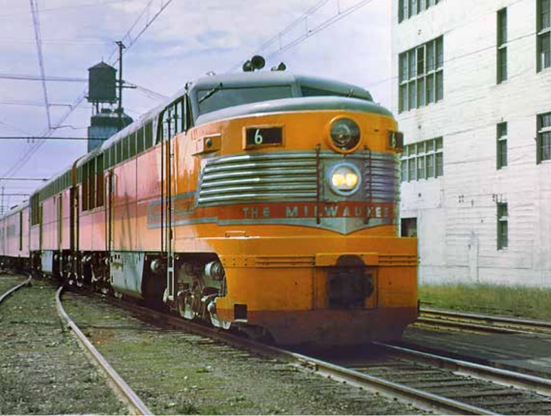
Initially, stylish Fairbanks-Morse “Erie-built” diesels powered the Olympian Hi through from Chicago to Seattle (where No. 6 was photographed). In 1949, GE and Westinghouse motors took over on the two electric districts, with steam in between. Dan Pope collection
