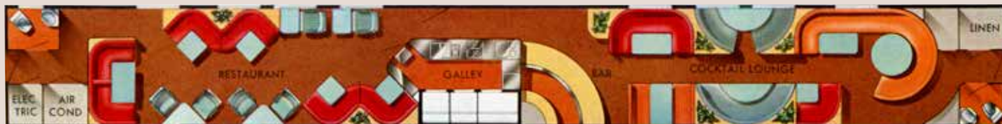
The tap-grill cars had seats for 18 in the dining area, 26 in the lounge. Like most Olympian Hi cars, the Milwaukee built them itself.
