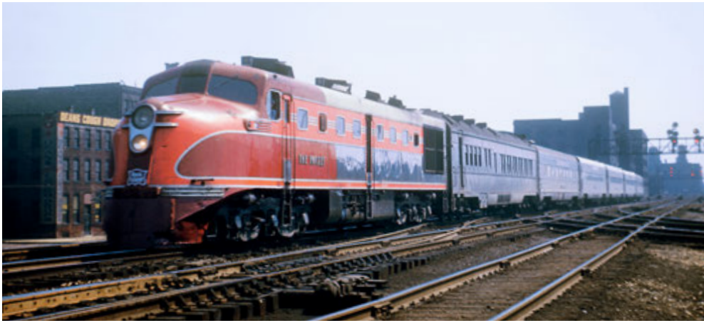
Diesel 624, the prototype for Alco-GE's line of "DL109" 2,000 h.p. passenger units, nears La Salle Street Station, Chicago, with the daily Rocket from Des Moines in fall 1946.
