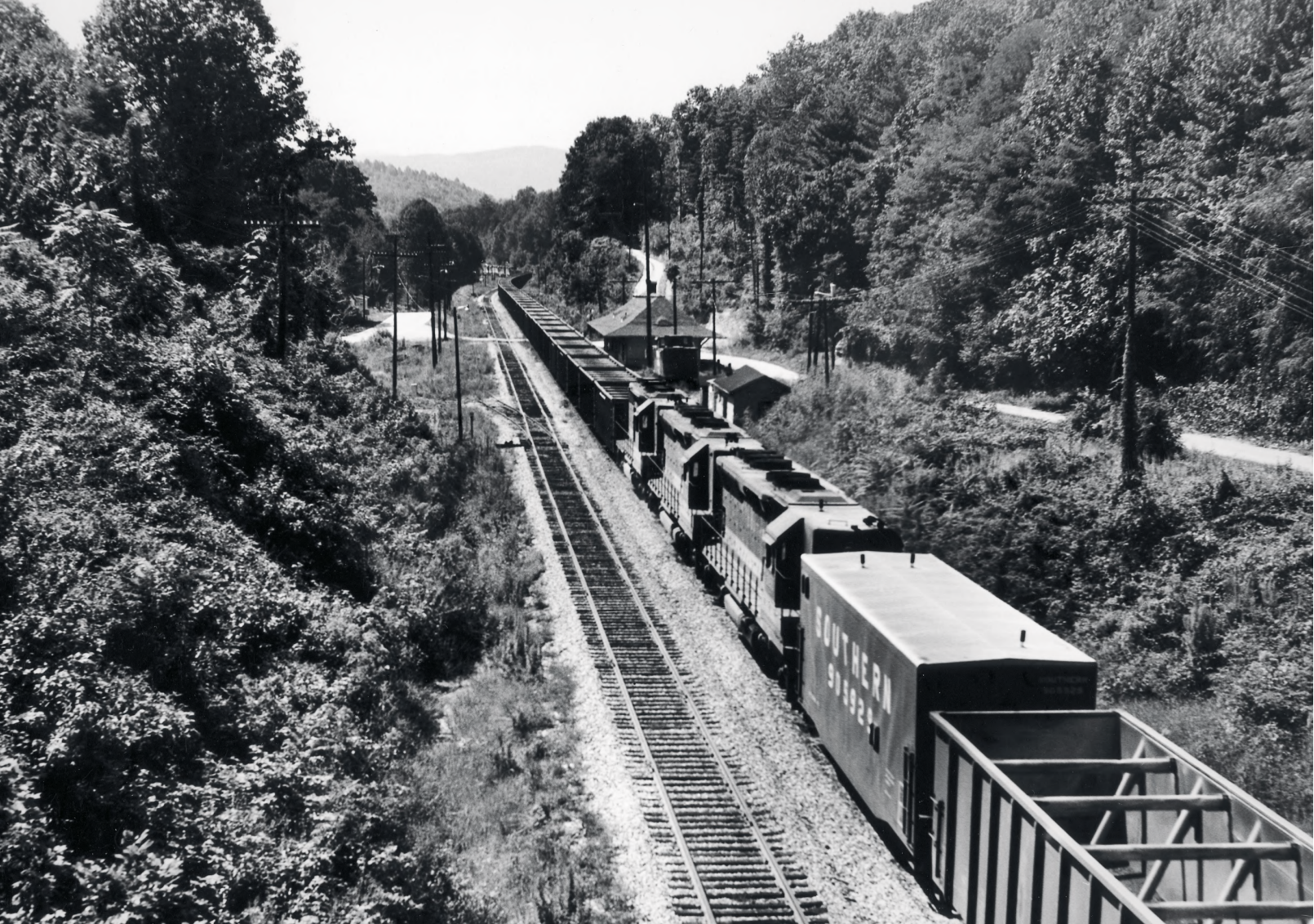
Forty-two years separate these views west from the U.S. Highway 176 bridge at Saluda. In 1938 (left), 2-8-8-2 4055 storms toward the crest of the hill with a train out of Asheville. In 1980, the mid-train "slave" units of an empty coal train approach the depot while the head-end units round a curve in the distance.
