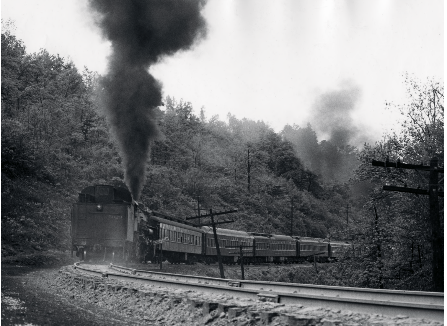
On the 10-degree curve just above Sand Cut, 2-10-2 No. 5029 shoves on the rear of the Carolina Special in April 1947. The angled sign to the right of the engine indicates that the switch for Safety Track No. 1 is 800 feet ahead. Specially modified for the hill, class Ss engines were Saluda fixtures until the end of steam.
