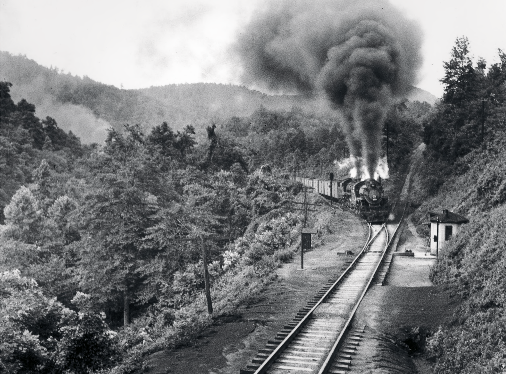
Two heavy Mikados, author Clodfelter's favorite Southern freight power, labor past Safety Track No. 1 with a train of reefers filled with peaches in the mid-1940s; smoke from a 2-10-2 pusher rises above the trees at left. This spur, considered superfluous in the diesel age, would be removed in the early 1950s.
