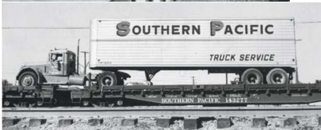
Trailers are loaded and unloaded "circus style" by means of a ramp at the end of track and retractable bridge plates between the flatcars. Once in place, the trailers are secured with cable tie-downs. Top, SP; others, Robert Hale
