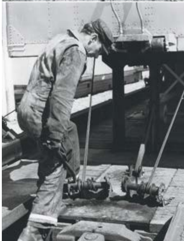
Trailers are loaded and unloaded "circus style" by means of a ramp at the end of track and retractable bridge plates between the flatcars. Once in place, the trailers are secured with cable tie-downs. Top, SP; others, Robert Hale
